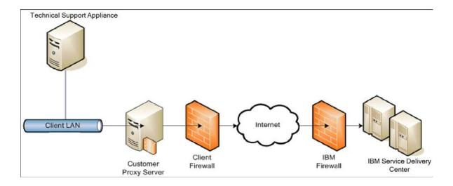
To forward packets, the proxy server must support the basic proxy header functions (as described in RFC #2616) and the CONNECT method. Optionally, basic proxy authentication (RFC #2617) may be configured so that TSA authenticates before attempting to forward packets through your proxy server.
