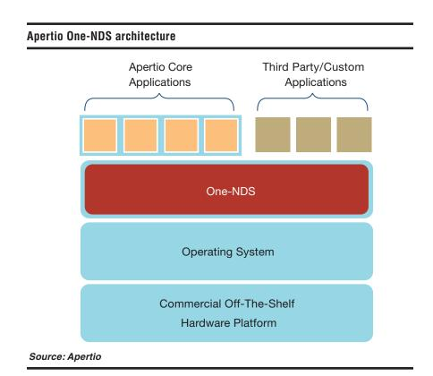
As services converge, the underlying infrastructure is also converging onto a common COTS based platform
