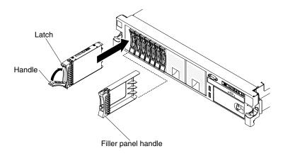
Figure 27. 2.5-inch hot-swap hard disk drives installation
