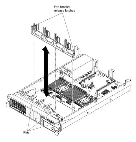
Figure 189. Fan bracket removal
