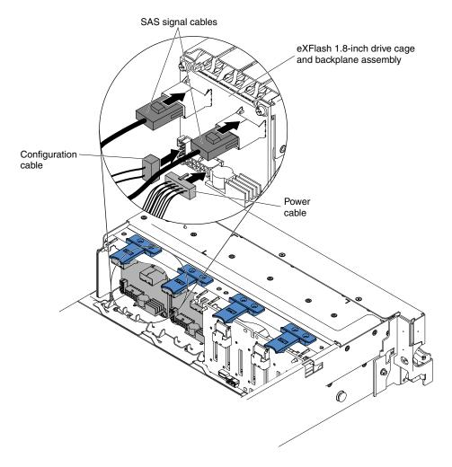
Figure 100. Cable connections
