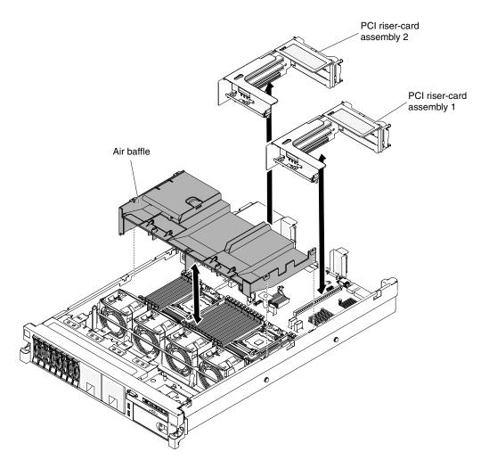
Figure 155. Air baffle installation
