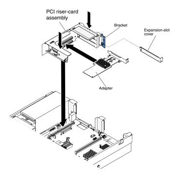
Figure 111. PCI riser-card assembly installation
