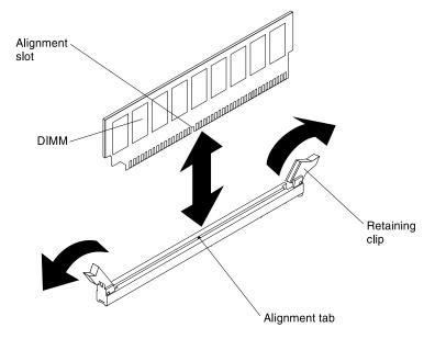
Figure 42. DIMM removal
