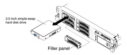
Figure 169. 3.5-inch simple-swap hard disk drive installation
