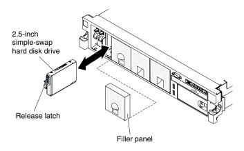
Figure 29. 2.5-inch simple-swap hard disk drive installation
