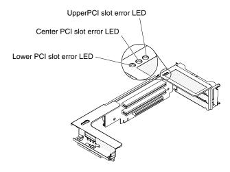
Figure 145. PCI riser-card LEDs
