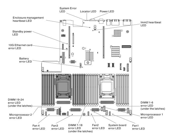
Figure 18. System-board LEDs
