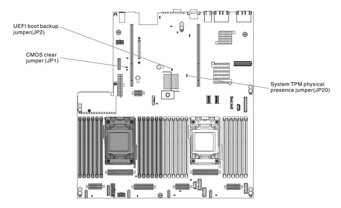
Figure 138. System-board switches, jumpers, and buttons
