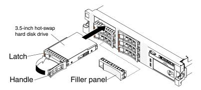
Figure 28. 3.5-inch hot-swap hard disk drives installation
