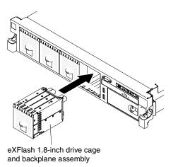
Figure 108. New backplane assemblies installation
