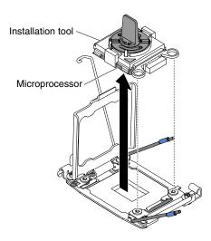
Figure 242. Installation tool removal
