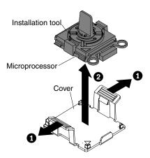
Figure 123. Installation tool cover removal
