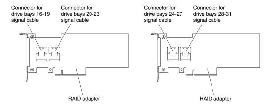
Figure 110. RAID adapter connectors
