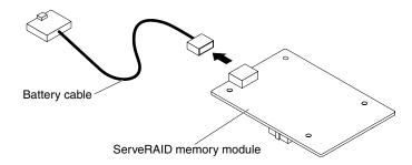
Figure 198. Disconnecting the battery cable
