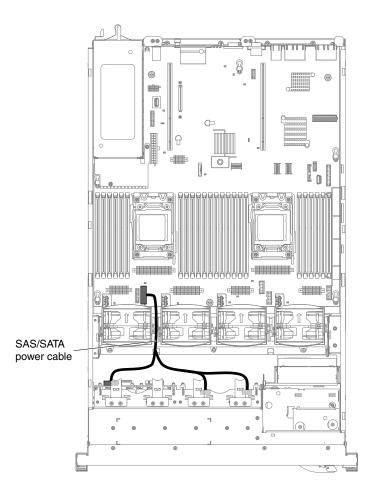
Figure 106. SAS/SATA power cable routing
