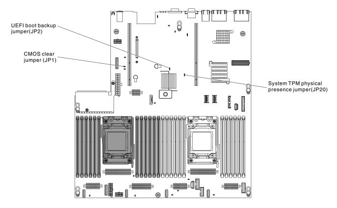
Figure 17. System-board switches, jumpers, and buttons
