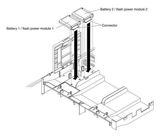
Figure 208. RAID adapter battery/flash power module installation
