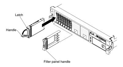
Figure 164. 2.5-inch hot-swap hard disk drives installation
