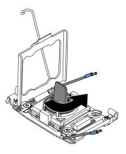
Figure 125. Installation tool handle adjustment
