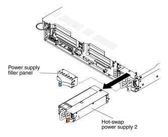
Figure 213. Power supply removal
