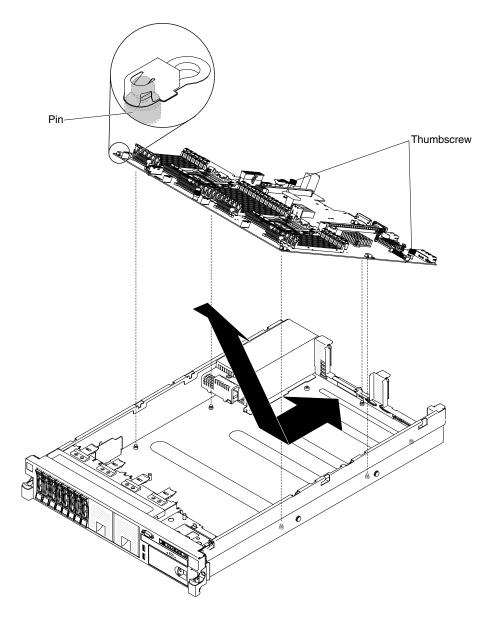
Figure 259. System board installation
