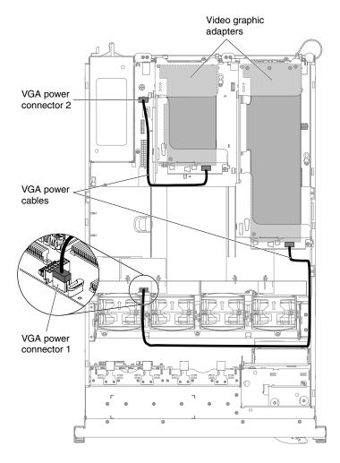
Figure 151. VGA power cables connection
