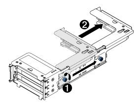
Figure 25. Stretching a PCI riser-card assembly
