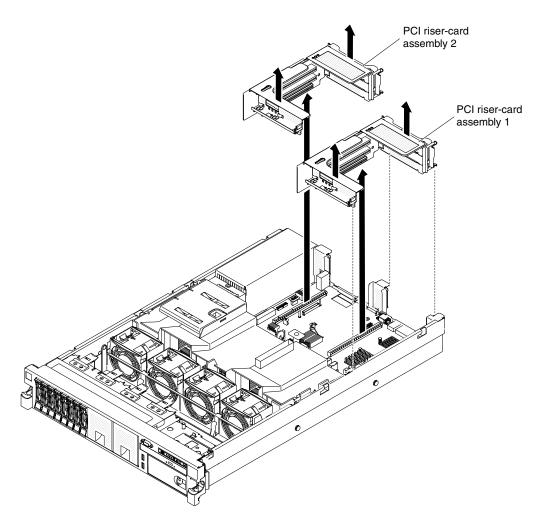
Figure 23. Removing PCI riser-card assembly
