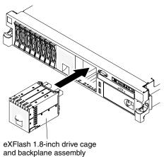
Figure 99. New backplane assemblies installation
