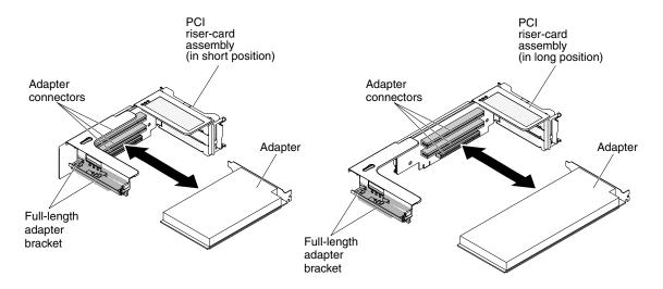
Figure 43. PCI riser-card adapter connectors
