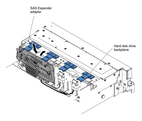
Figure 72. New backplane installation
