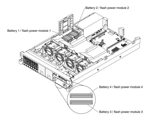
Figure 206. RAID adapter battery/flash power module installation
