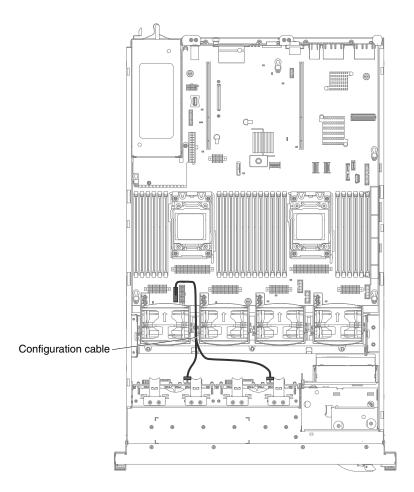
Figure 75. Configuration cable routing
