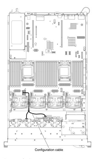
Figure 68. Configuration cable routing
