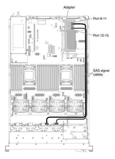
Figure 74. Mini-SAS signal cables routing
