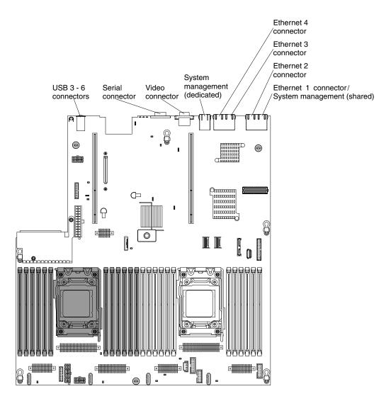
Figure 16. System-board external connectors
