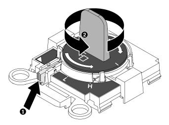
Figure 239. Installation tool handle adjustment
