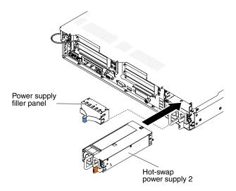
Figure 218. Power supply installation
