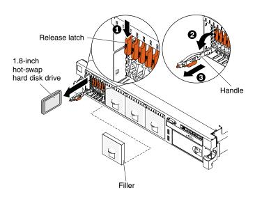
Figure 170. 1.8-inch hot-swap solid state drives removal
