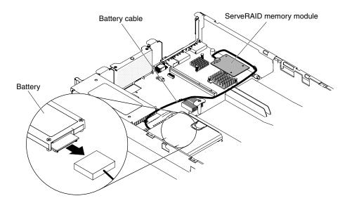
Figure 195. Disconnecting the battery cable
