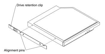
Figure 33. DVD drive retention clip installation
