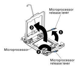
Figure 237. Microprocessor socket levers and retainer disengagement
