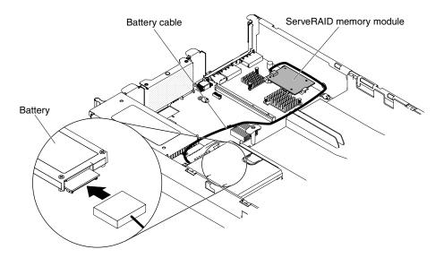
Figure 50. Connecting the supercap cable
