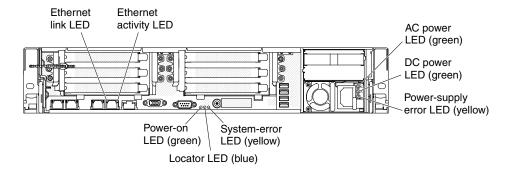
The following illustration shows the LEDs on a dc power supply.
