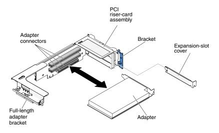
Figure 44. Adapter installation
