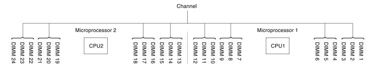
Figure 39. Connectors on each memory channel
