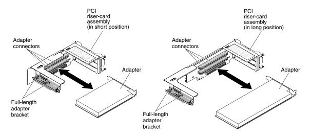
Figure 20. PCI riser-card adapter connectors
