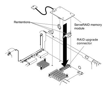
Figure 49. Installing ServeRAID upgrade adapter and supercap cable
