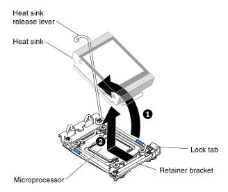
Figure 236. Heat sink removal
