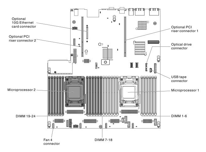
Figure 19. System-board optional-device connectors
