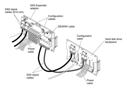
Figure 65. Cables connection
