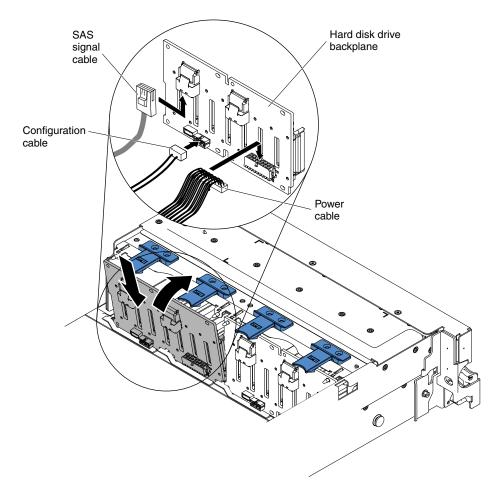
Figure 86. New backplane installation
