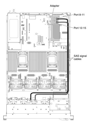
Figure 103. SAS signal cables routing
