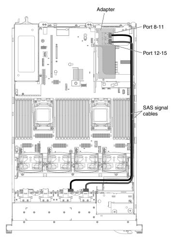
Figure 88. Mini-SAS signal cables routing
