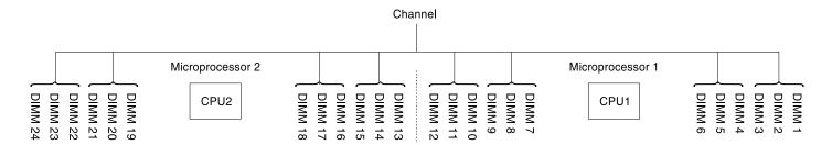
Figure 186. Connectors on each memory channel
