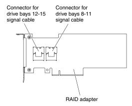
Figure 80. RAID adapter (part number 00D7082)
