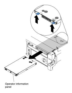
Figure 233. Operator information panel removal
