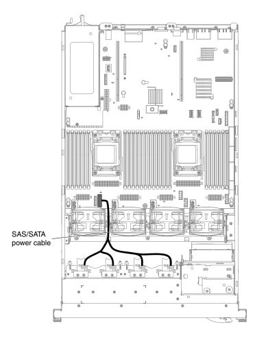
Figure 115. SAS/SATA power cable routing
