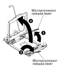
Figure 245. Microprocessor socket levers and retainer disengagement
