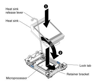
Figure 253. Heat sink installation
