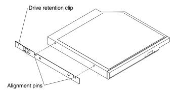
Figure 174. DVD drive retention clip installation
