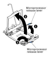
Figure 122. Microprocessor socket levers and retainer disengagement
