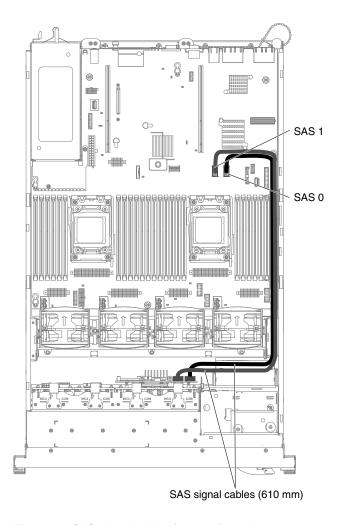
Figure 67. SAS signal cables (610 mm) routing
