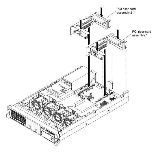
Figure 134. Installing a PCI riser-card assembly
