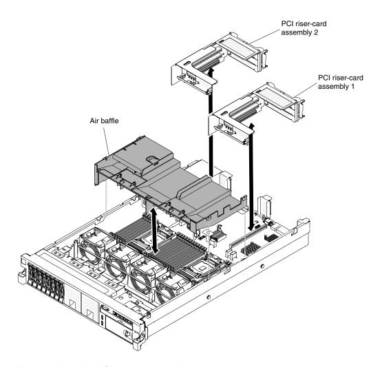
Figure 41. Removing PCI riser-card assembly
