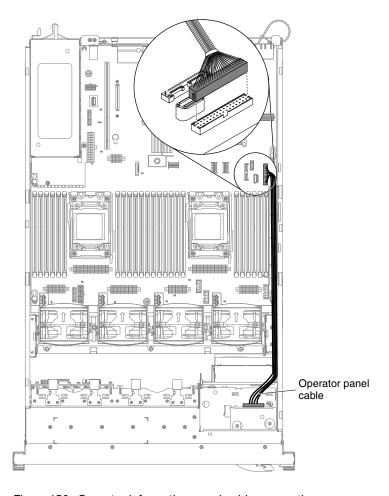
Figure 150. Operator information panel cable connection
