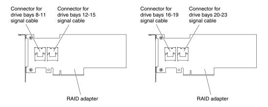
Figure 101. RAID adapter connectors
