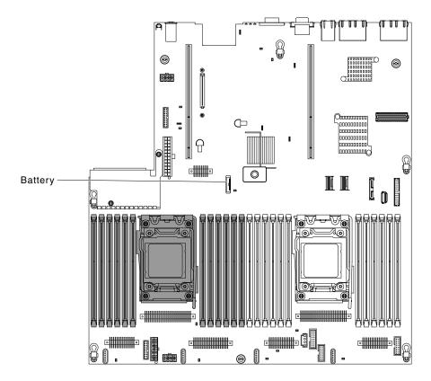
Figure 229. System battery removal
