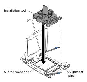
Figure 240. Installation tool alignment
