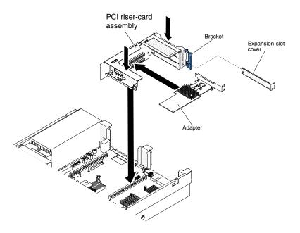
Figure 87. PCI riser-card assembly installation
