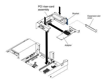
Figure 102. PCI riser-card assembly installation
