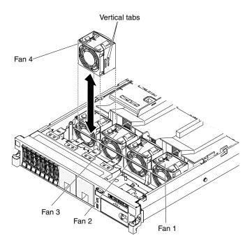
Figure 221. Fan removal
