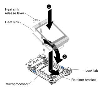
Figure 130. Heat sink installation
