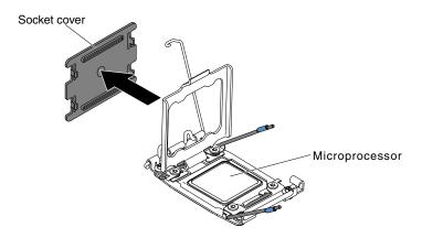
Figure 127. Socket cover removal
