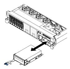
Figure 180. Tape drive removal
