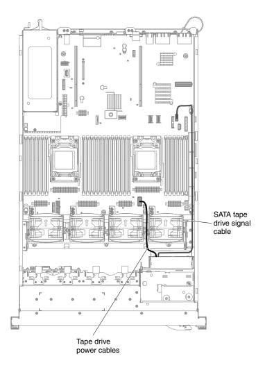
Figure 118. Cable connections
