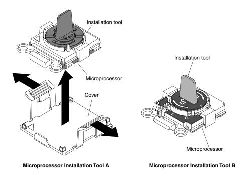
Figure 120. Microprocessor installation tools
