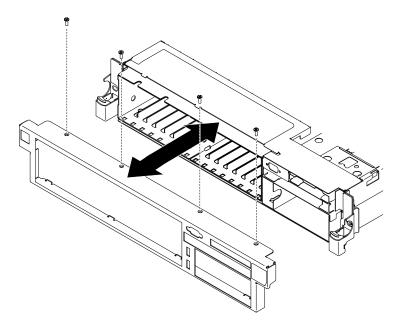
Figure 159. Bezel installation
