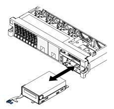
Figure 116. Tape drive installation
