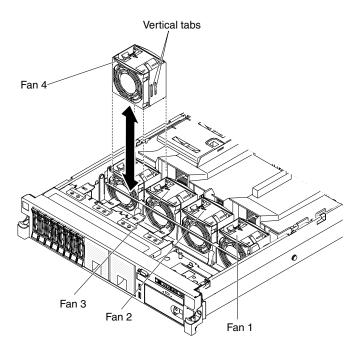
Figure 62. Fan installation
