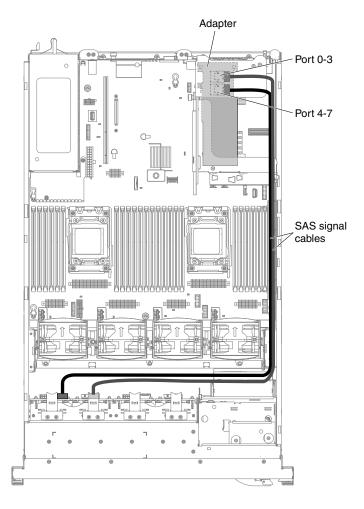
Figure 96. SAS signal cables routing
