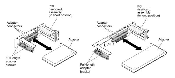
Figure 193. Adapter removal
