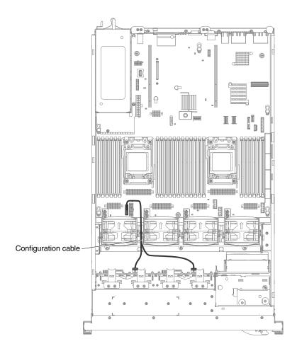
Figure 83. Configuration cable routing
