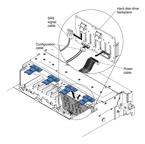
Figure 64. Hard disk drive backplane removal
