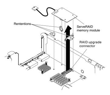
Figure 197. Removing ServeRAID upgrade adapter memory module
