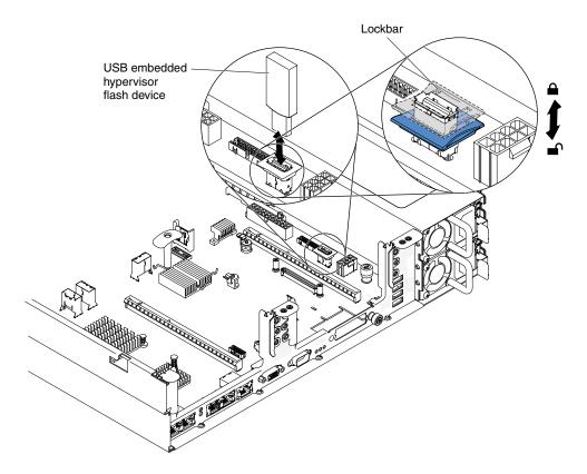
Figure 119. USB hypervisor flash device installation
