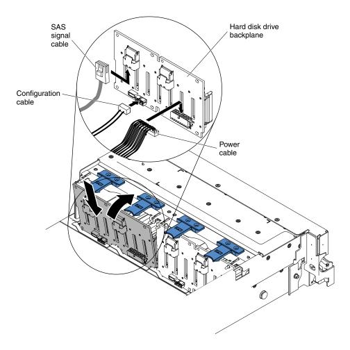
Figure 78. New backplane installation
