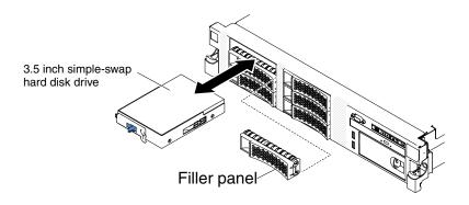
Figure 30. 3.5-inch simple-swap hard disk drive installation
