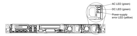
Figure 143. AC power-supply LEDs
