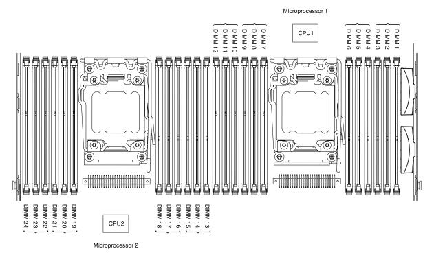
Figure 185. DIMM connectors location
