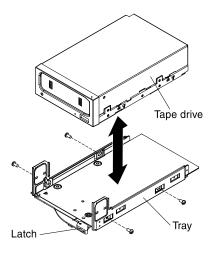
Figure 117. Installing the tape drive on the tray
