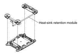
Figure 256. Heat-sink retention module removal
