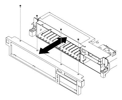
Figure 158. Bezel removal
