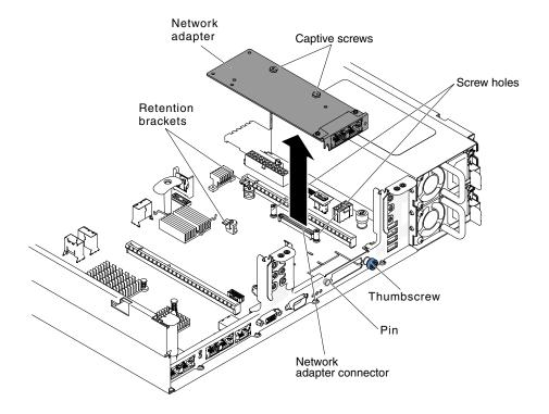
Figure 210. Screws disengagement
