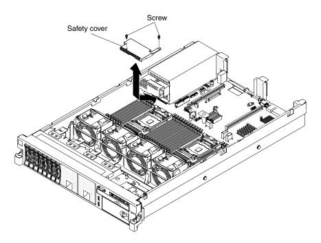
Figure 161. 240 VA safety cover installation
