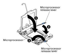
Figure 128. Microprocessor socket levers and retainer engagement
