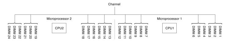
Figure 40. Connectors on each memory channel
