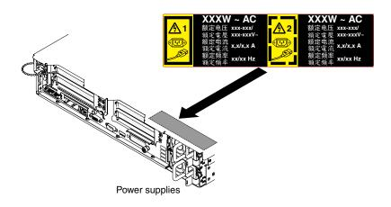
Figure 57. Attaching the redundant power information label
