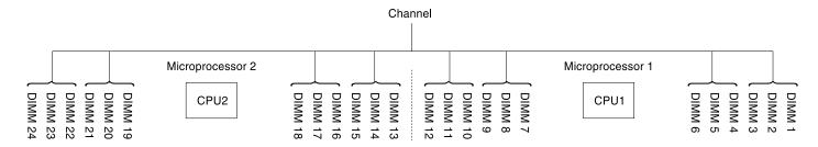
Figure 187. Connectors on each memory channel
