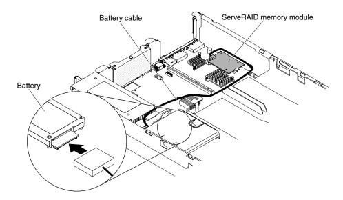
Figure 203. Connecting the battery cable
