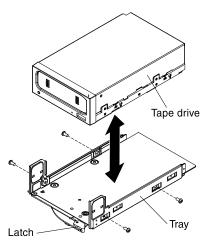
Figure 181. Screws removal
