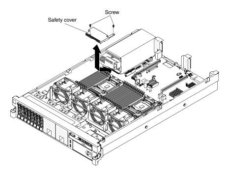
Figure 160. 240 VA safety cover removal
