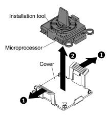
Figure 246. Installation tool cover removal
