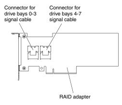
Figure 94. RAID adapter connectors
