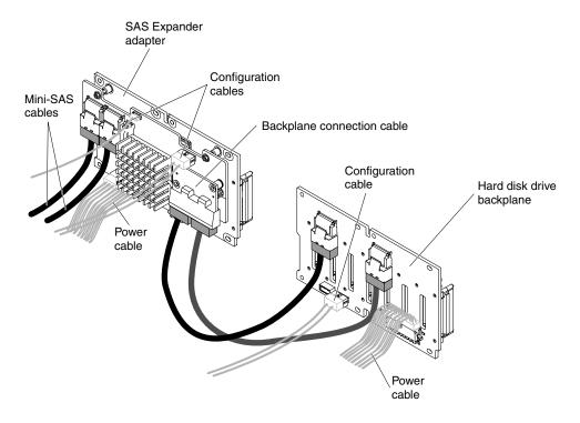
Figure 71. Cables connection
