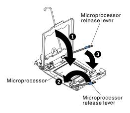
Figure 251. Microprocessor socket levers and retainer engagement
