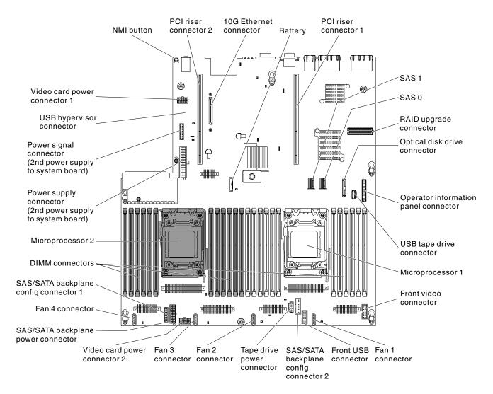
Figure 15. System-board internal connectors
