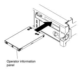
Figure 234. Operator information panel installation
