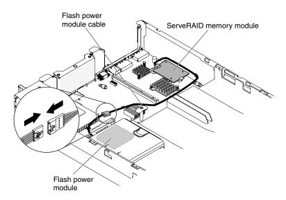
Figure 204. Connecting the flash power module cable
