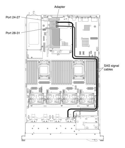
Figure 113. SAS signal cables routing
