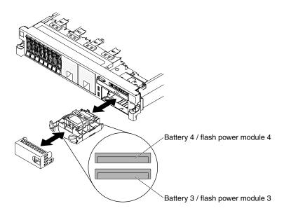
Figure 156. RAID adapter battery holder removal
