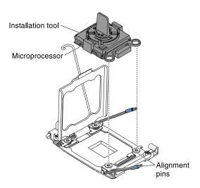
Figure 247. Installation tool alignment
