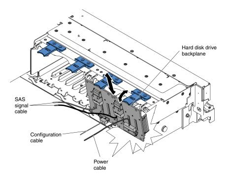
Figure 224. 2.5-inch simple-swap/hot-swap hard disk drive backplate assembly/backplane installation
