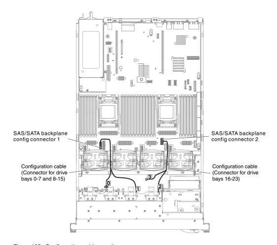
Figure 105. Configuration cables routing
