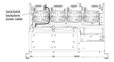
The following illustration shows the cabling information for the hardware RAID cable in the server:
