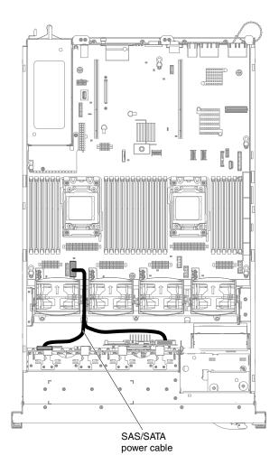
Figure 69. SAS power cable routing
