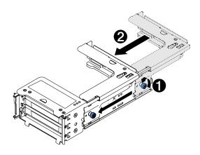
Figure 26. Shrinking a PCI riser-card assembly
