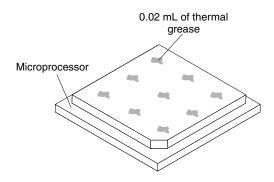
Figure 131. Thermal grease distribution
