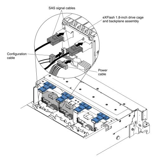
Figure 109. Cable connections
