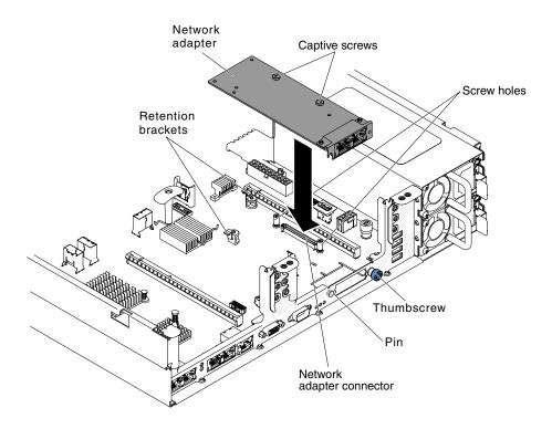
Figure 212. Network adapter installation
