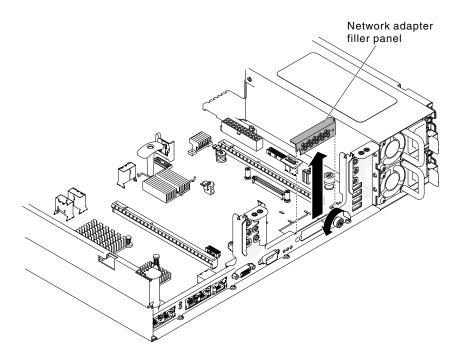
Figure 53. Adapter filler panel removal
