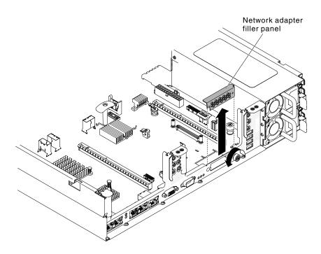
Figure 211. Adapter filler panel removal
