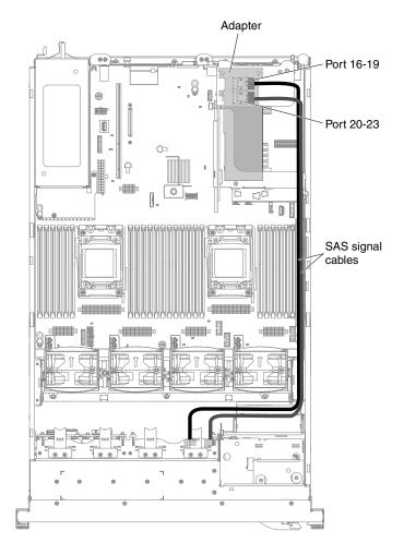
Figure 104. SAS signal cables routing
