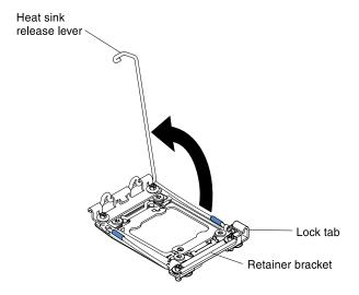
Figure 244. Heat-sink lever rotation
