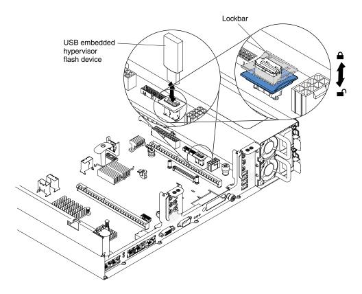
Figure 228. USB hypervisor flash device installation
