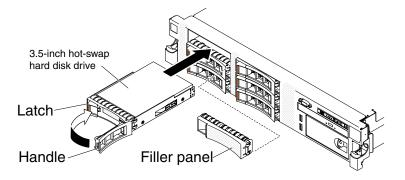
Figure 165. 3.5-inch hot-swap hard disk drives installation
