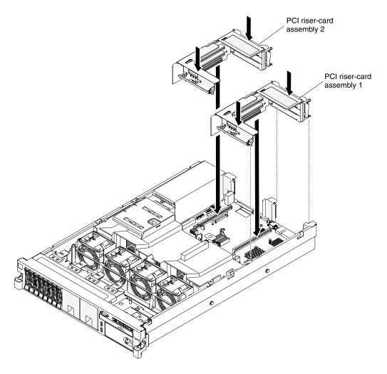
Figure 47. Installing PCI riser-card assembly
