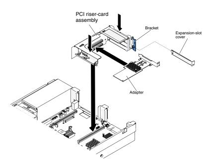
Figure 73. PCI riser-card assembly installation
