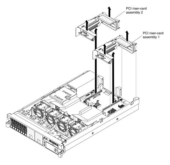
Figure 191. Removing PCI riser-card assembly
