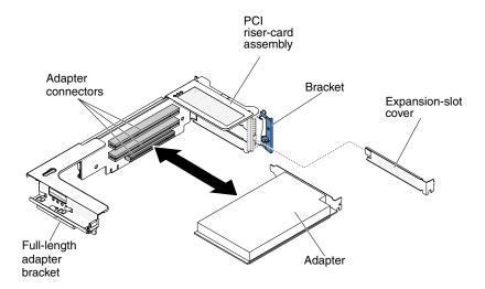
Figure 194. Adapter installation
