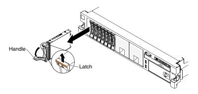
Figure 162. 2.5-inch hot-swap hard disk drives removal
