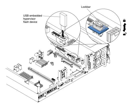
Figure 227. USB hypervisor flash device removal
