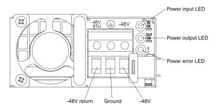
Figure 217. DC power supply rear view
