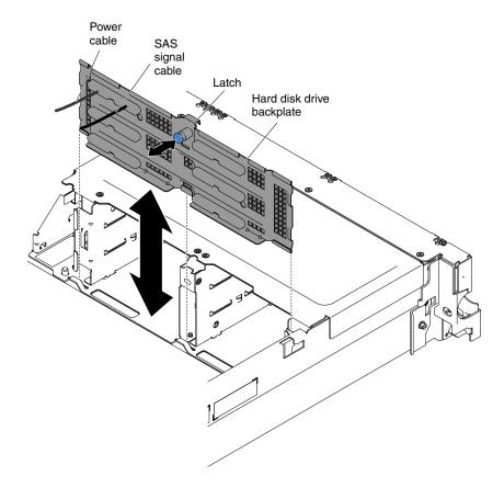
Figure 225. 3.5-inch simple-swap/hot-swap hard disk drive backplate assembly/backplane removal
