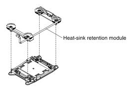
Figure 257. Heat-sink retention module installation
