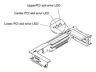
Figure 21. PCI riser-card assembly LEDs
