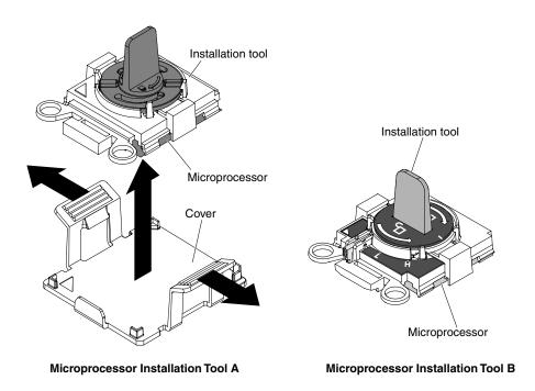
Figure 243. Microprocessor installation tools
