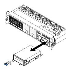
Figure 183. Tape drive installation
