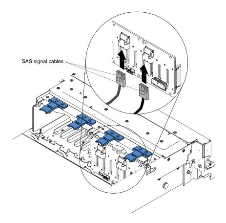
Figure 93. SAS cables connection
