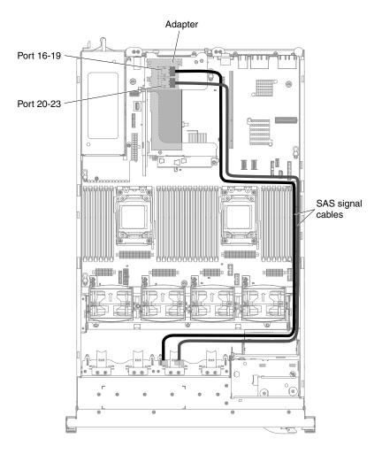
Figure 112. SAS signal cables routing
