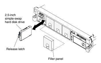
Figure 168. 2.5-inch simple-swap hard disk drive installation
