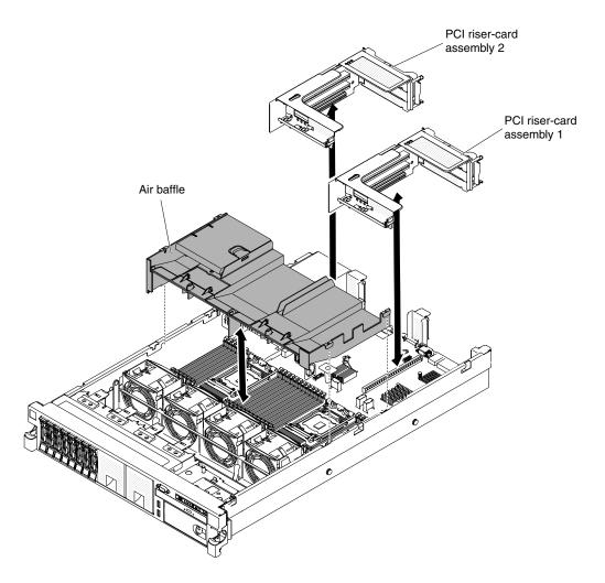
Figure 24. Air baffle removal
