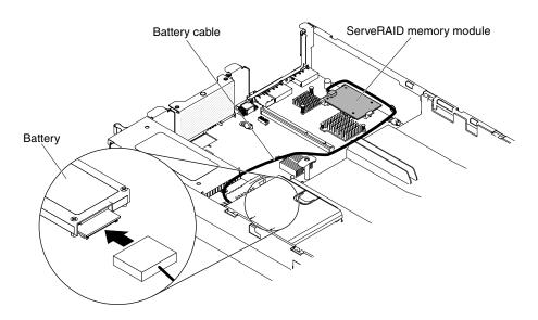
Figure 209. RAID adapter battery/flash power module installation
