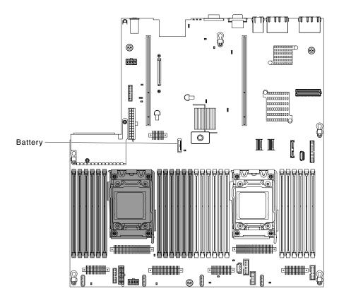
Figure 231. System battery installation
