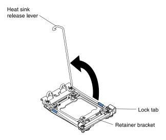
Figure 121. Heat-sink lever rotation
