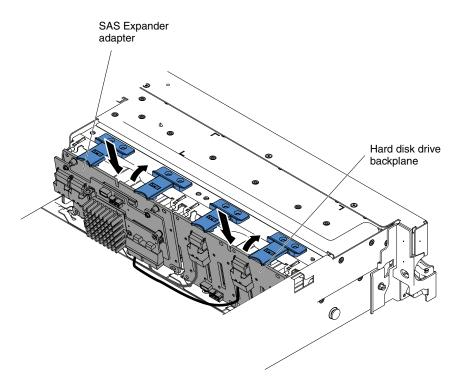
Figure 66. New backplane installation
