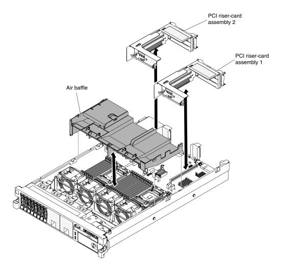
Figure 154. Air baffle removal
