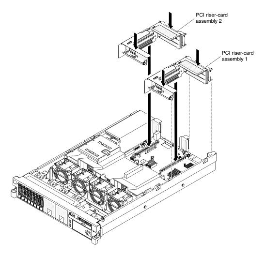
Figure 192. PCI riser-card assembly installation
