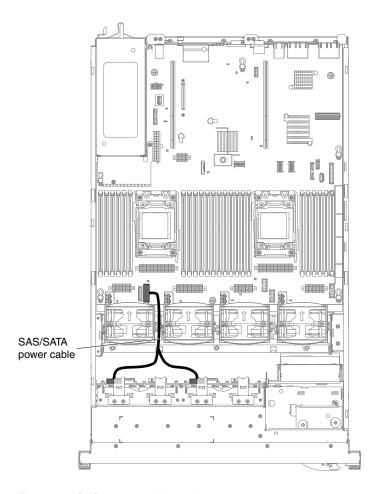
Figure 90. SAS power cable routing
