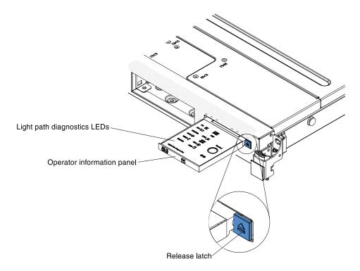
Figure 140. Light path diagnostics panel disengagement
