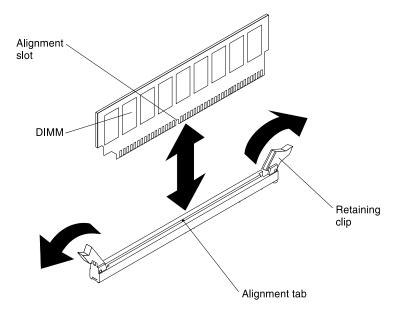
Figure 188. DIMM installation
