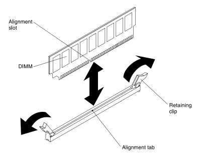
Figure 184. DIMM removal
