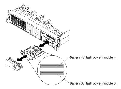
Figure 207. RAID adapter battery/flash power module installation
