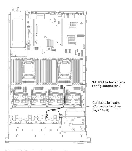
Figure 114. Configuration cables routing
