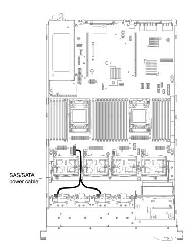
Figure 76. SAS power cable routing
