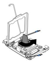
Figure 248. Installation tool handle adjustment
