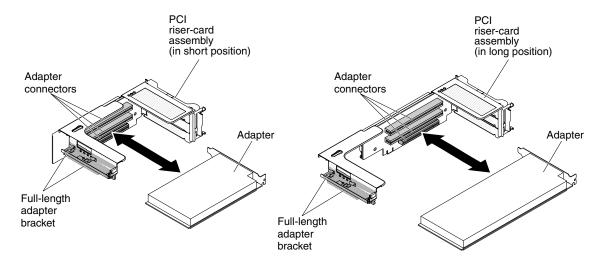
Figure 46. PCI riser-card adapter connectors
