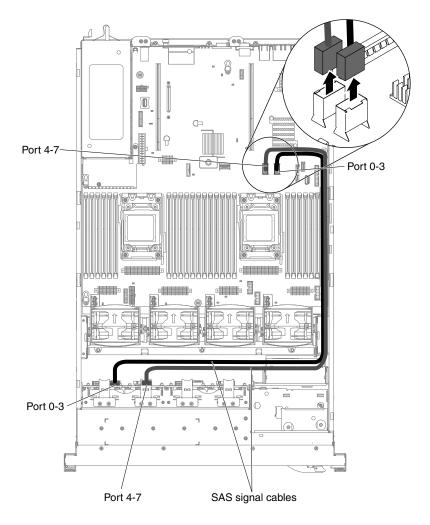
Figure 92. SAS cables removal
