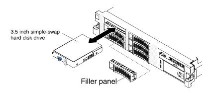
Figure 167. 3.5-inch simple-swap hard disk drive removal
