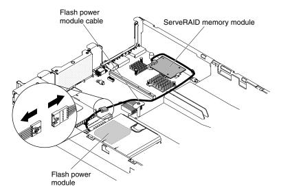
Figure 196. Disconnecting the flash power module cable
