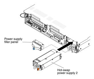
Figure 55. Power supply installation
