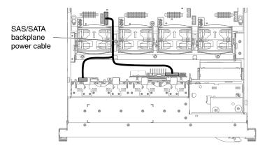
The following illustration shows the cabling information for the hardware RAID cable in the server:
