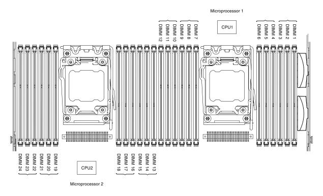
Figure 38. DIMM connectors location
