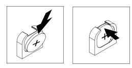
Figure 232. System battery installation
