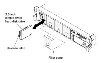
Figure 166. 2.5-inch simple-swap hard disk drive removal
