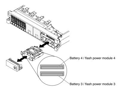
Figure 157. RAID adapter battery holder installation
