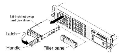
Figure 163. 3.5-inch hot-swap hard disk drives removal
