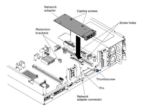
Figure 54. Network adapter installation
