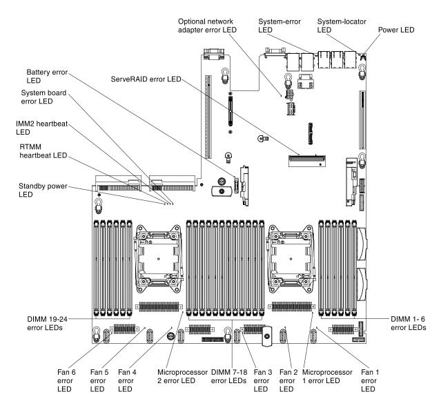
Figure 142. System board error LEDs
