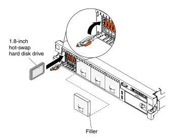
Figure 31. 1.8-inch hot-swap solid state drives installation
