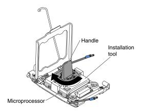
Figure 241. Installation tool handle adjustment
