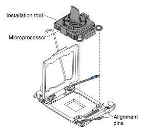
Figure 124. Installation tool alignment
