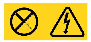
Hazardous voltage, current, and energy levels are present inside any component that has this label attached. There are no serviceable parts inside these components. If you suspect a problem with one of these parts, contact a service technician.
