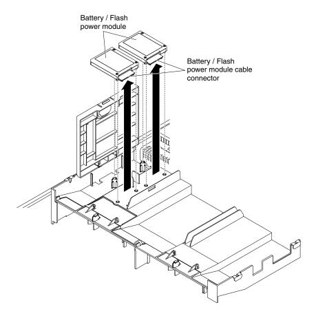
Figure 205. RAID adapter battery/flash power module removal
