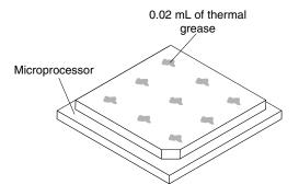
Figure 254. Thermal grease distribution
