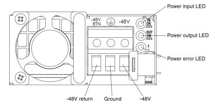
Figure 144. DC power-supply LEDs
