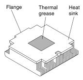
Figure 129. Thermal grease
