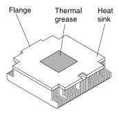
Figure 252. Thermal grease
