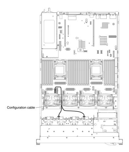
Figure 89. Configuration cable routing
