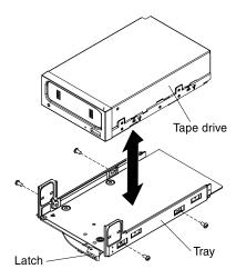
Figure 182. Screws installation
