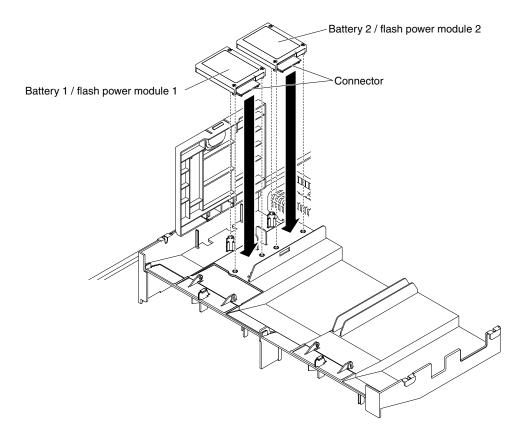
Figure 52. RAID adapter battery installation
