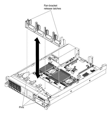
Figure 190. Fan bracket removal
