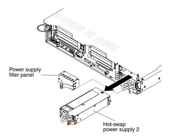
Figure 216. Power supply removal
