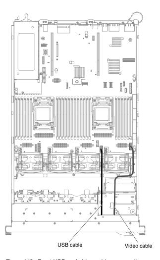
Figure 149. Front USB and video cables connection
