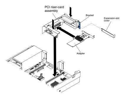
Figure 81. PCI riser-card assembly installation
