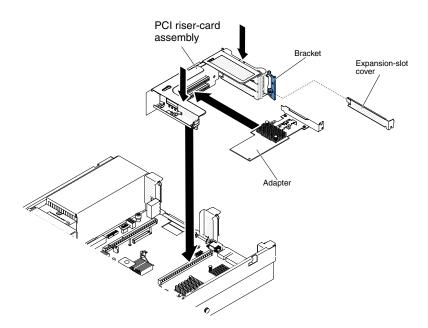
Figure 95. PCI riser-card assembly installation
