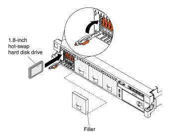
Figure 171. 1.8-inch hot-swap solid state drives installation
