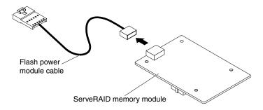
Figure 199. Disconnecting the flash power module cable
