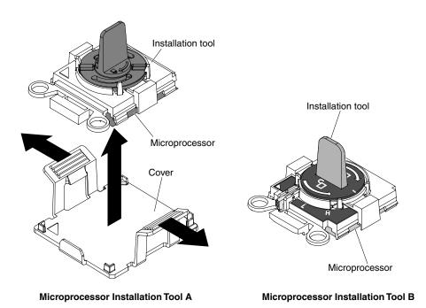
Figure 235. Microprocessor installation tools
