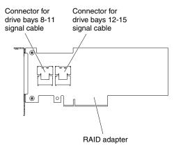
Figure 79. RAID adapter (part number 46M0912)
