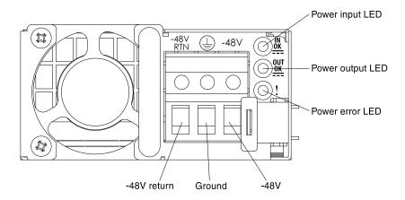
Figure 58. DC power supply rear view
