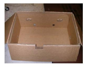
2.5 Place corrugated clip (6X) (37L0511) into square holes in bottom tray and snap shut. Insure that clips go through carton and tray securing carton and tray together.
