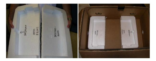
2.8 Place system inside bag (6165640) and place system in bottom cushions. Make sure the system is positioned all the way down and not sitting on the cushion ledge.
