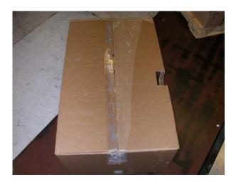
2.13 Check the parts list for additional carton label which are called out. If there is a Processor-related label ("Intel" or "AMD"), place the appropriate label on the top of the carton between the label location marks. If there is no processor-related label on the parts list, leave this area on the carton blank.
