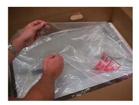
2.9 Fold system bag over unit and seal edges of bag closed with Tamper label (06P6550).
