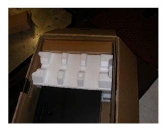
2.12 Close the top of the carton and seal using printed tape (74F5699 - Automatic taper, 74F5698 - for hand held dispensers).
