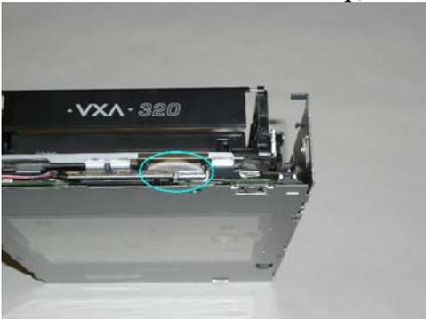
Once the stack in the tape is taken up by turning the white gear toward the right, continue turning the screw with the Philips screwdriver in the clockwise direction as outlined in step 4 until you see the slack tape build up again as the tape guides move toward the front of the drive. Repeat steps 4 and 5 until the you see the cartridge start to raise up and the cartridge loader begin to move forward towards the front of the drive.
