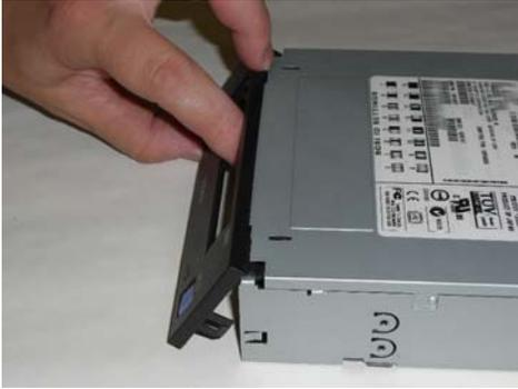
**IMPORTANT!** You will need to keep the door open until the bezel has been fully seated to be sure that the door is positioned behind the door opening mechanism.
