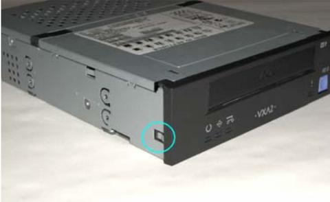
2. Now open up the bezel by rotating it upwards towards the tape drive's top and remove it from the tape drive, disengage it from the upper tabs of the tape drive chassis and remove the bezel.
