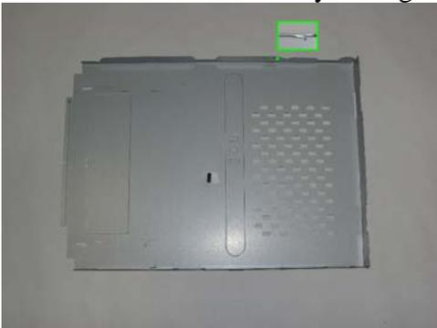
3. In order to disengage and remove the tape cartridge itself the metal bar – highlighted in the green frame - in the tape drive must be moved towards the end of the tape drive.
