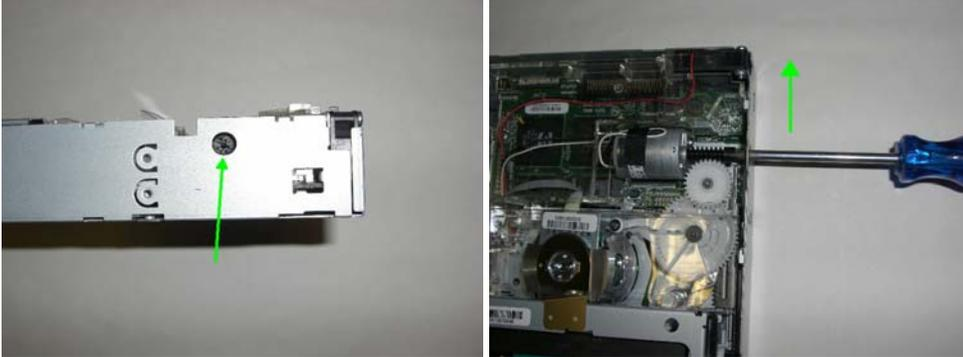
Observe that the tape guides also are slowly moving in their slots toward the front of the drive which is removing tension from the tape and creating slack tape. **Stop turning the screw.**
