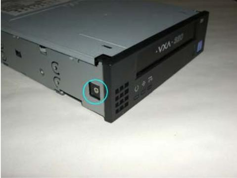
2. Rotate the bezel upwards towards the tape drive's top. Disengage it from the upper tabs of the tape drive chassis and remove the bezel.
