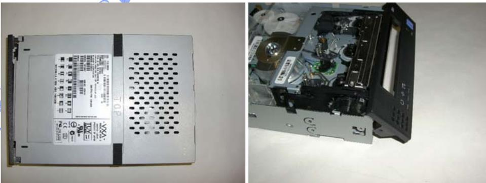
2. Slowly rotate the bezel down until it engages with the tape drive's chassis and also lines up correctly with the tape drive's chassis bottom. Make sure the holes in the chassis align with the holes on the bezel sides.
