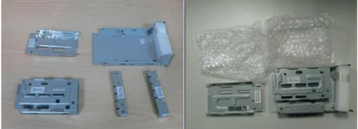
2.3 - Place wrapped metal brackets into carton P/N 75H8621.
