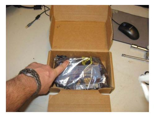
2.9 - Flip the divider over on top of the bagged cage, shut the tuck-lock and seal with IBM logo tape P/N 46D2114.
