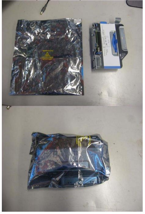
2.8 - Place the bagged riser cage in carton P/N 75H8621 making sure the printed circuit board side of the cage is on the side of the carton with the top flap.
