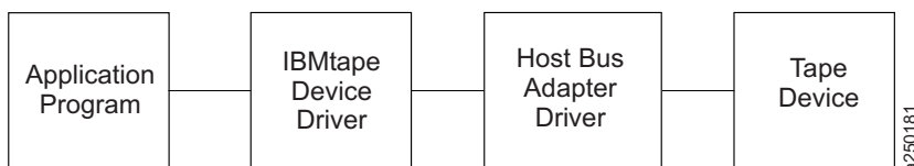
Figure 11. Data flow for Linux device driver (lin_tape)
