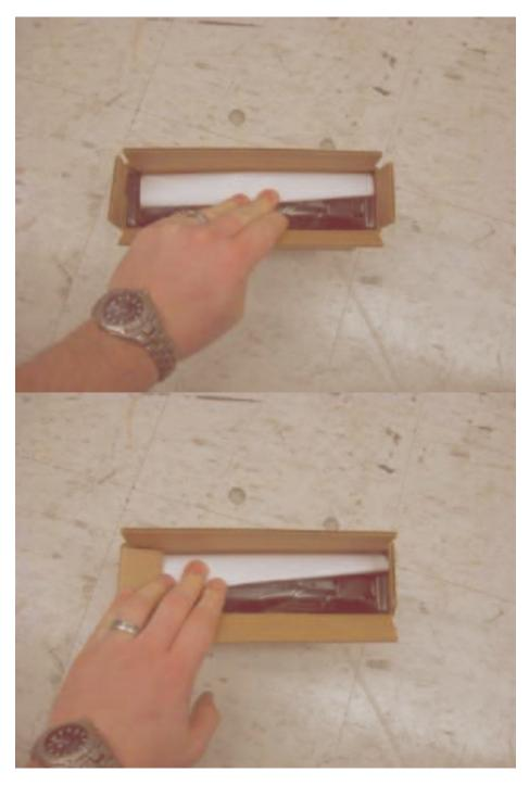
1.6 - Seal the top of the RSC shut with IBM logo tape P/N 46D2114
