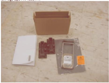
1.1 - Place HDD assembly in ESD P/N 4759223, fold bag and seal opening with ESD label P/N 6937292.
