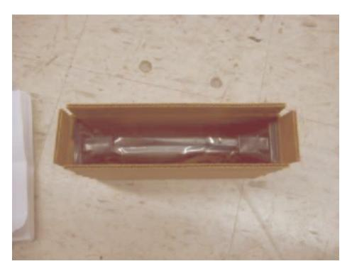
**1.4** - Grab for pubs, ensure the pubs are folded in half top to bottom, then slide the pubs down in between the carton side wall and the HDD.
