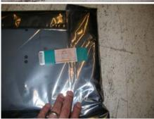
1.3 Locate front (44R4013) and rear (44R4014) cushions and place them onto blade unit as shown below. Please note that the latch/handles/connectors must line up with the slots on the cushions.
