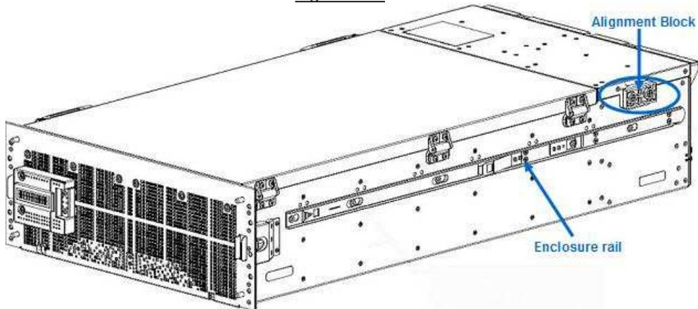
3. Attach the enclosure rails to each side of chassis by positioning the rails over the keyhole tabs, and slide the rails into place. The rails are marked "R" (right) and "L" (left) viewing from the front of the enclosure. Do not exchange the enclosure rails. Secure each rail using seven #8-32 flat head screws (Figure 15b).
