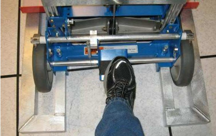
2. Carefully disengage the enclosure rails from the rack rails and slide the rack rail back into the rack (Figure 14a and 14b). The SS8460 Enclosure is now dismantled from the rack. Adjust Load plate up and down as necessary for ease of enclosure removal.
