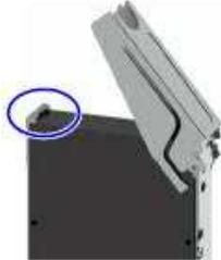
5. Carefully slide the module from the disk slot (Figure 11).
