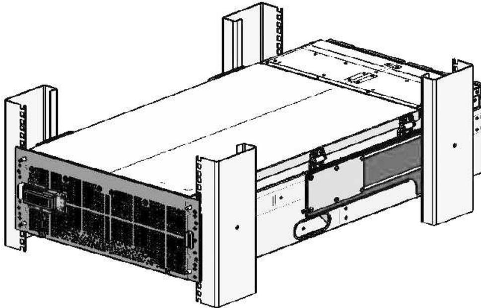
7. Carefully reinstall all drives removed in previous steps by sliding the module into a disk slot until it contacts the baseboard and begins to engage the handle (Figure 11). Press down on the handle until it latches which will cam the module into place.
