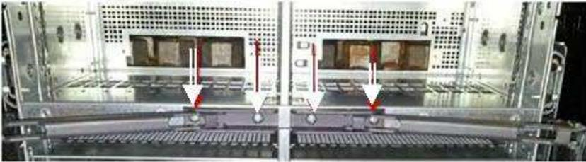
9. Remove the CMA cross bar on the rear panel of the enclosure by removing two #10-32 screws as shown in Figure 7.
