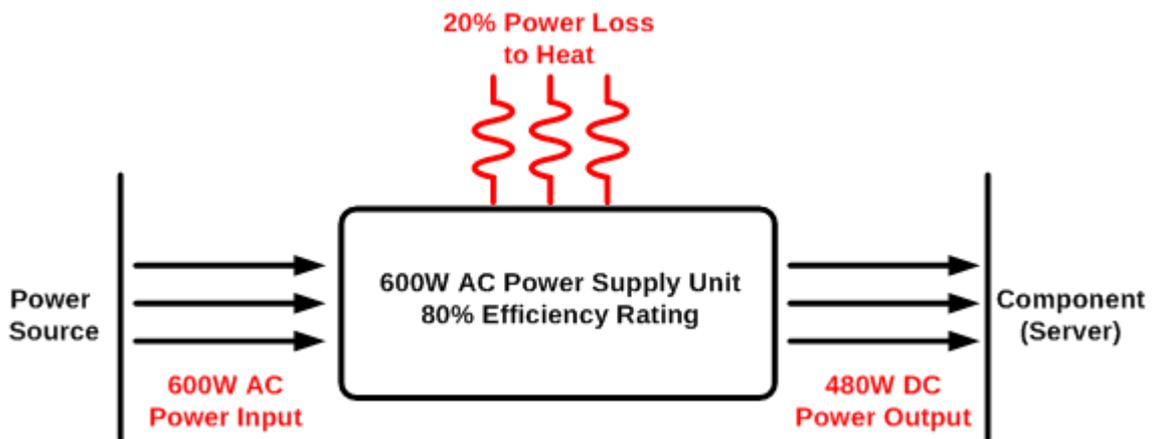
Figure 31: Simple example of Power Supply efficiency
