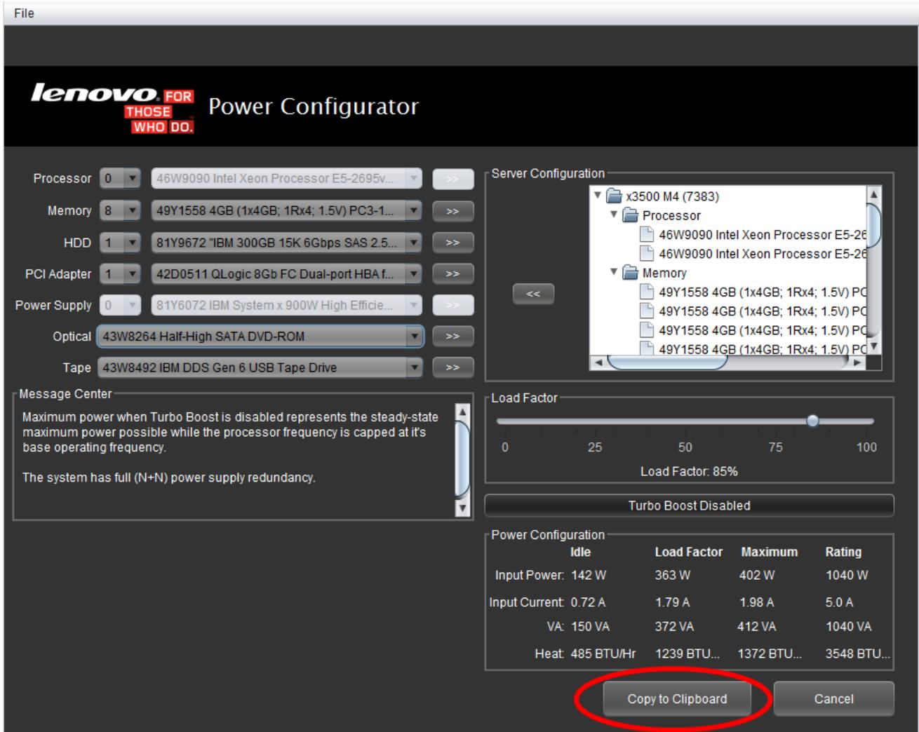
Figure 22: System x Power Configurator - copy to clipboard
