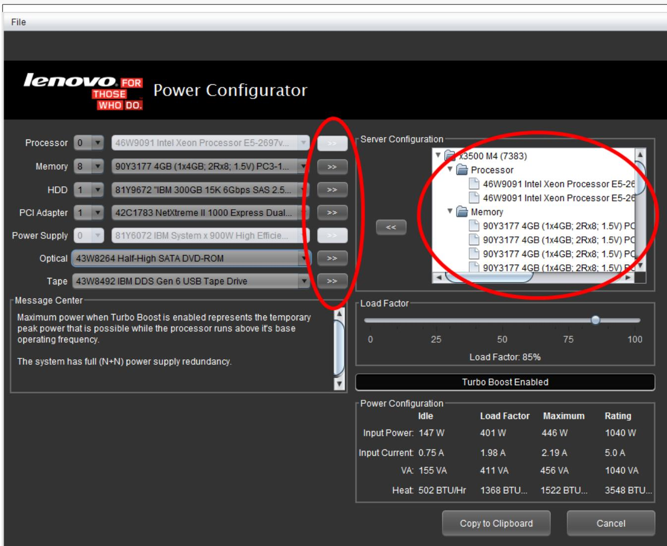
Figure 10: System x Power Configurator - Server Builder screen configuration example
