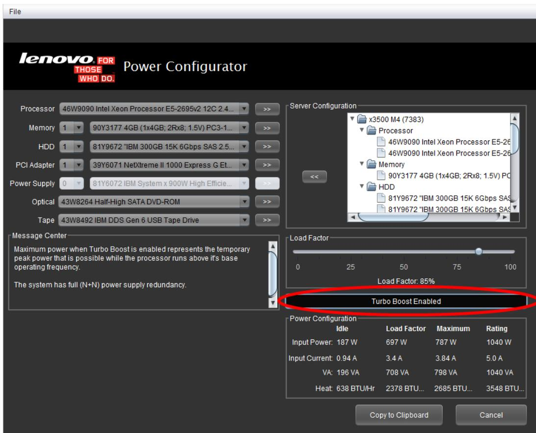
Figure 20: System x Power Configurator - Turbo Boost button
