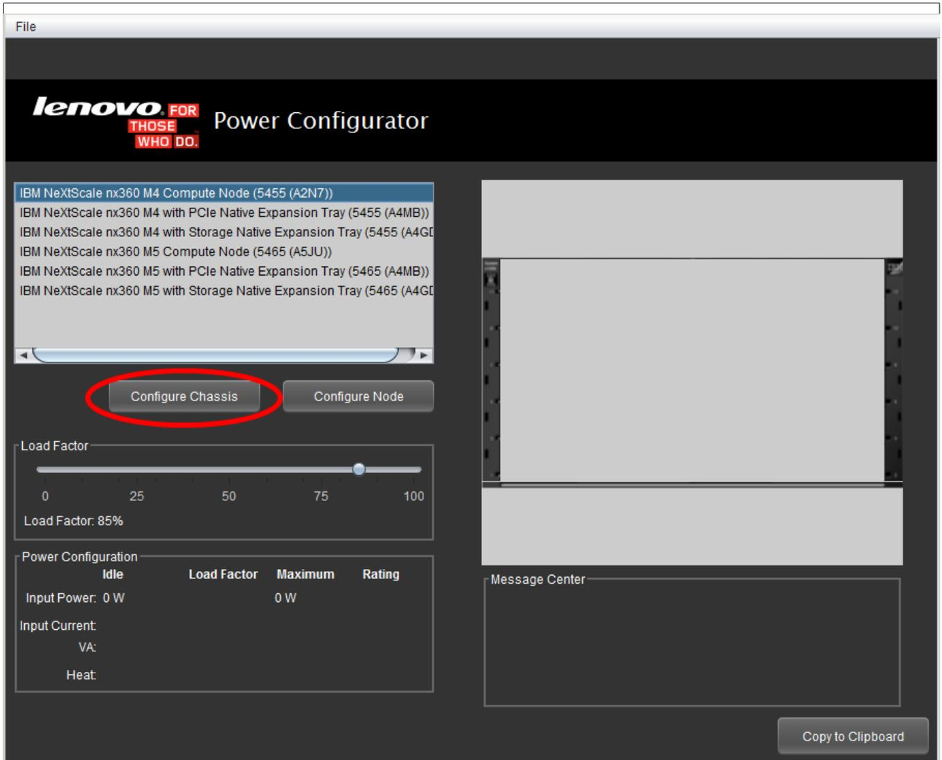
Figure 12: System x Power Configurator - Chassis Builder screen configuration example
