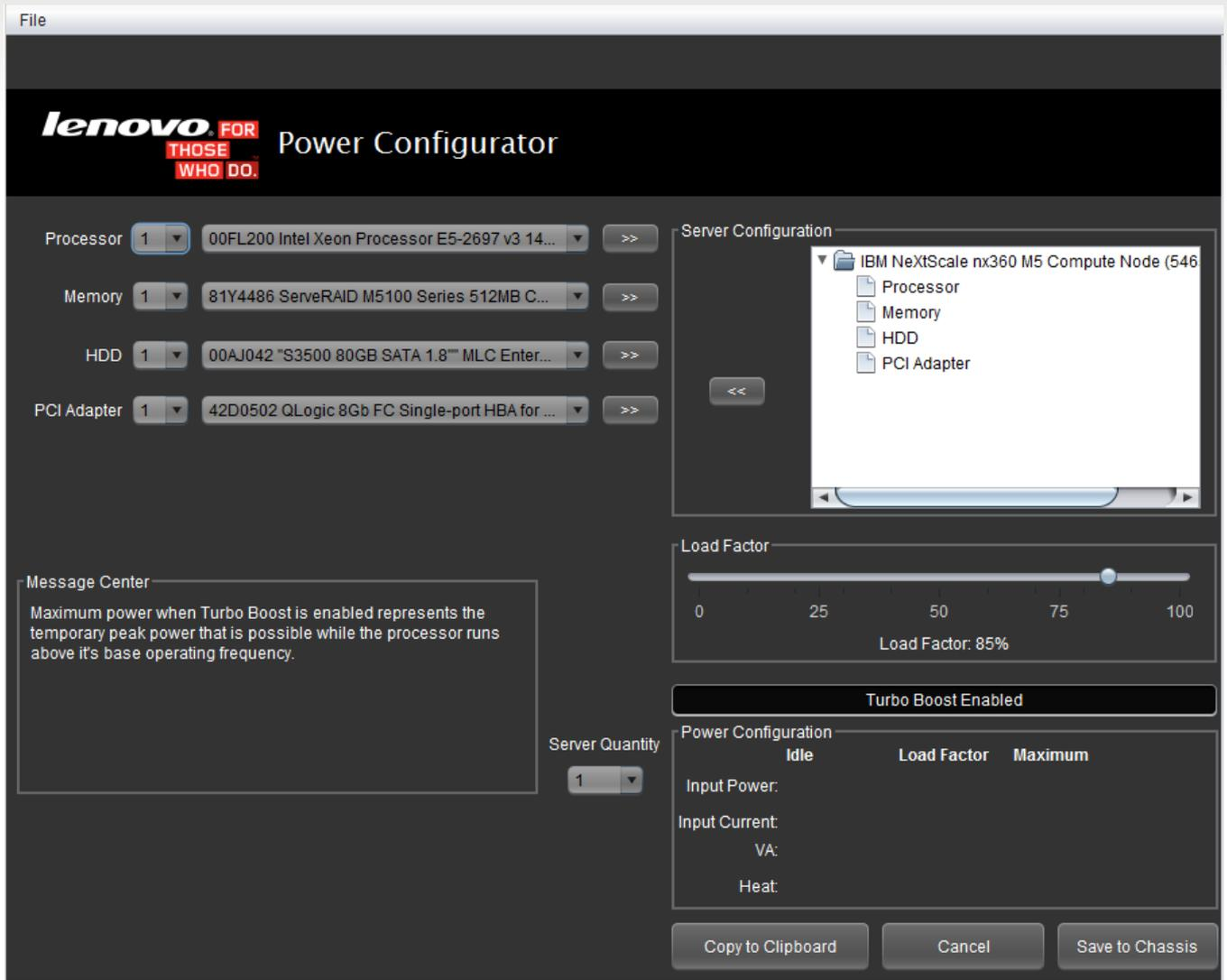
Figure 17: System x Power Configurator - Node Builder screen configuration example
