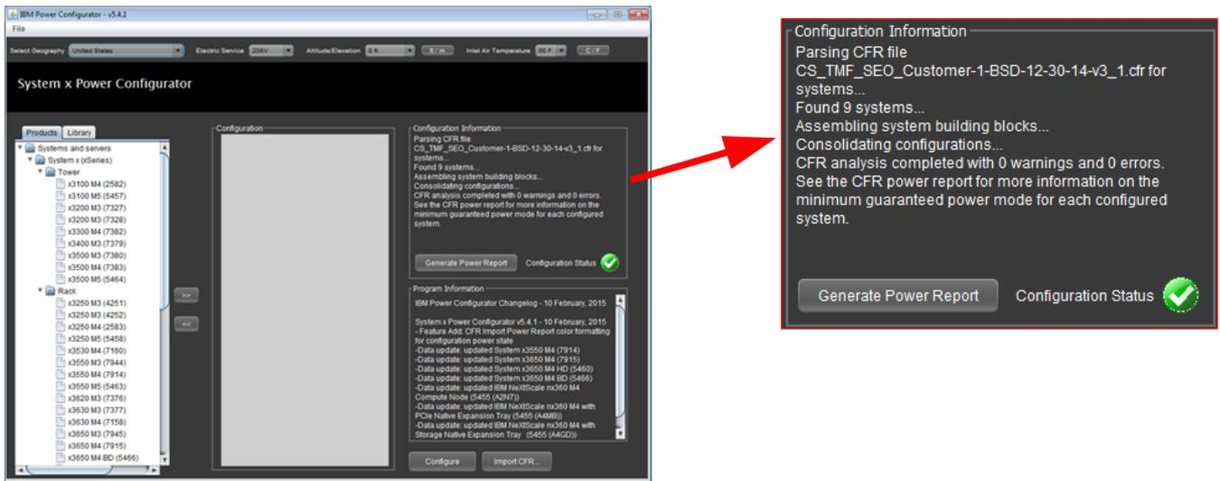
Figure 27: Configuration Information screen with imported CFR file
