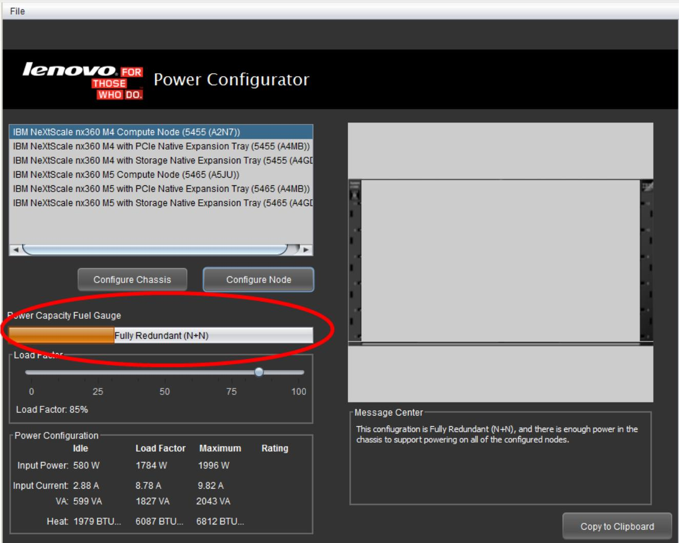
Figure 24: Power Capacity/Fuel Gauge indicator
