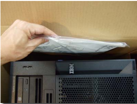
2.10 - Fold cardboard filler 43W4815 and insert it into the space at the bottom of chassis.
