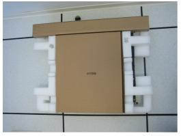
2.9 - Slide assembly bottom first into the carton.
