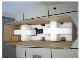
2.10 - Close flaps and seal carton as shown using IBM logo tape. Carton should be palletized standing upright with front facing up.
