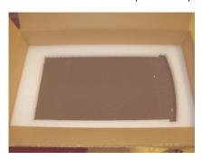
1.5 - Place corrugated loadspreader 22K8232 over the rear of the blade, outside of the ESD bag, as shown below and place into cushions.
