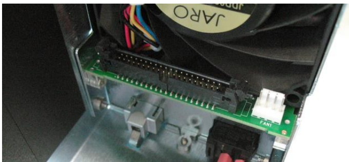
Figure 5.10: Removing the Front Fan Enclosure: The picture shows the power connector and ribbon cable removed.
