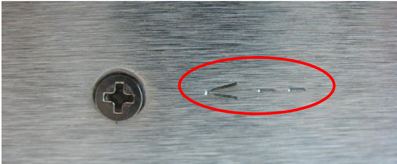
Figure 5.7 Removing the Top of the Canister: The only screws that need to be removed to access the canister are marked by arrows etched into the metal.
