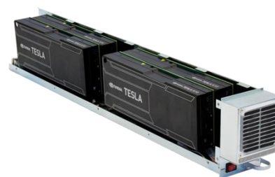
Figure 2.6 Four NVIDIA GPUs installed in a canister
