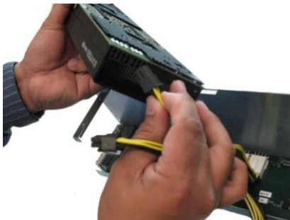
Figure 5.17: Removing the Auxiliary Power Cables from the GPU
