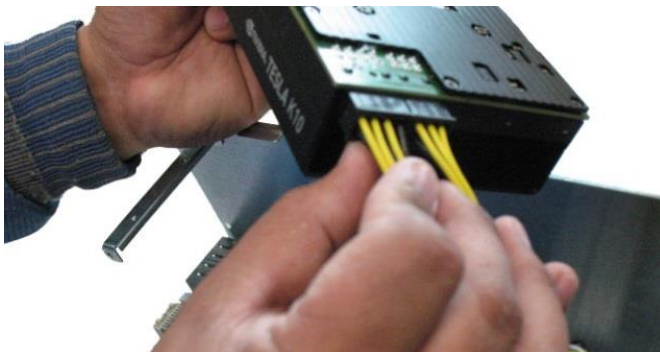
Figure 5.18: Inserting the Auxiliary Power Cables into the GPU
