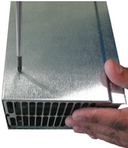
Figure 5.7.1 Removing the Top of the Canister: Unscrew 8 screws.
