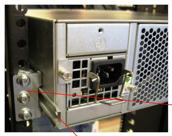
Rear rack mount bracket is attached to the rear of an iDataPlex rack
