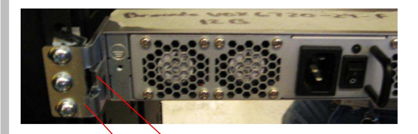
Rear rail mounted on switch slides into rear bracket
