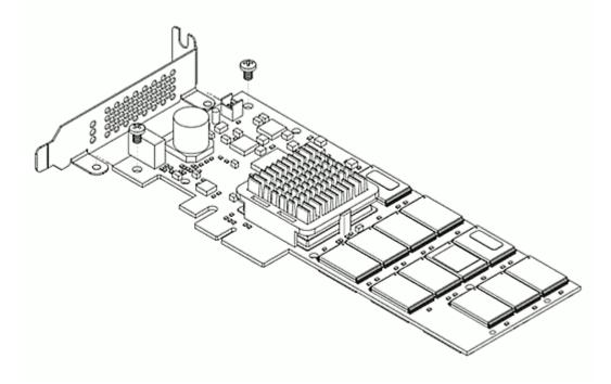
5. Attach the half-height bracket using a Phillips #1 tip screwdriver to tighten the two screws.
