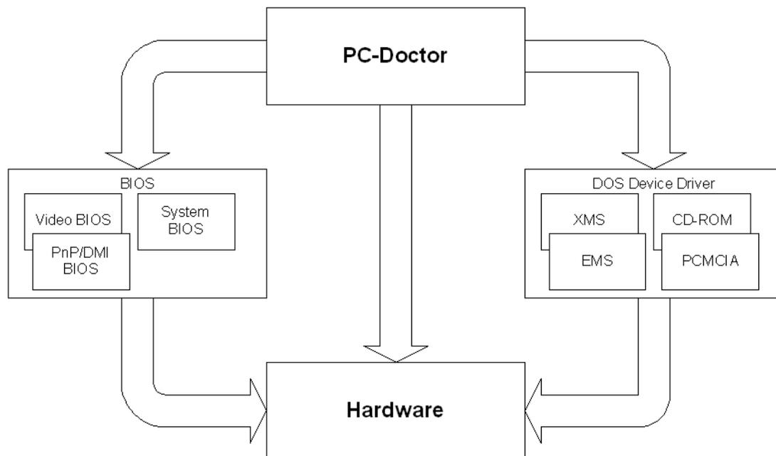
**Figure 1: Information Access Paths for PC-Doctor for DOS Components**
