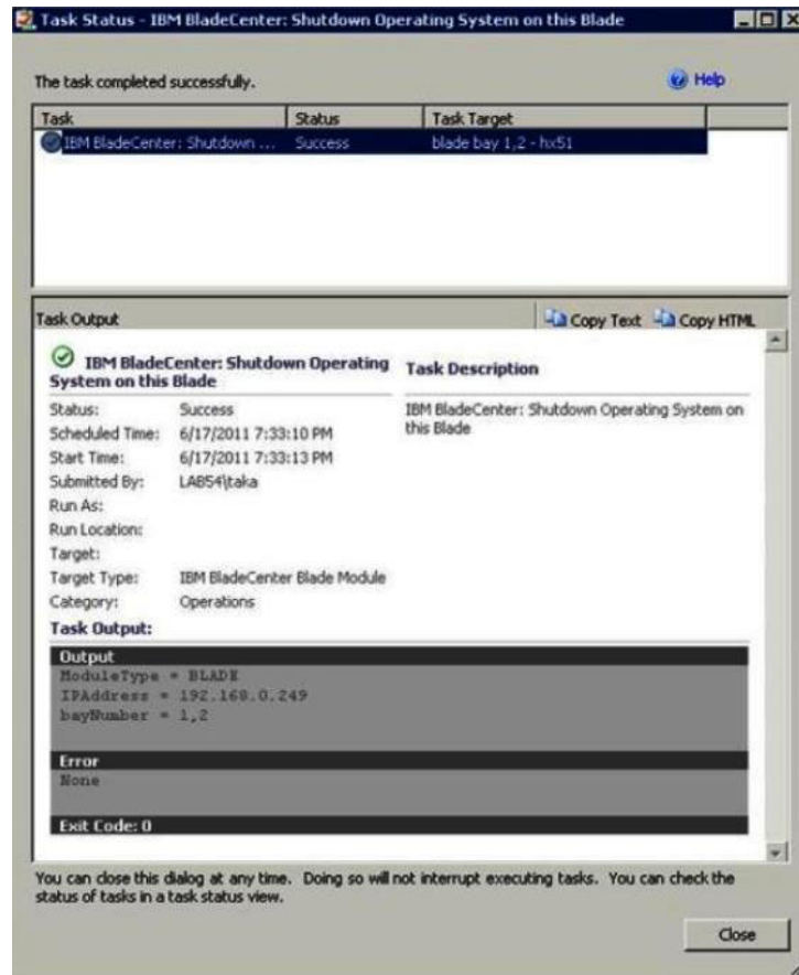
Figure 55. Task Status indicating the shutdown task has been sent to this Blade
