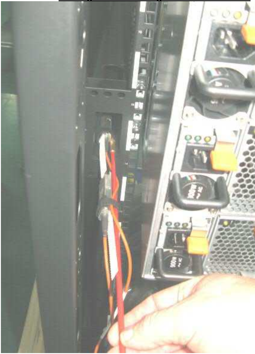
Fishing Cables Through Cable Channel #3
