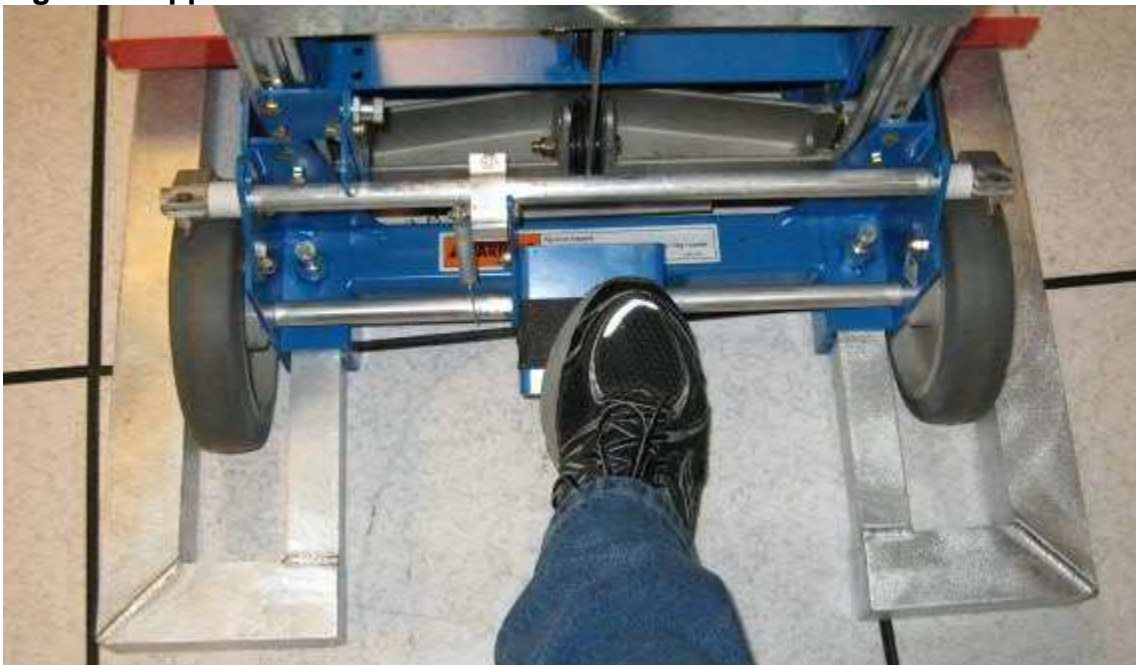
Figure 3. Application of lift tool break mechanism.
