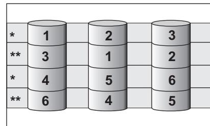
With RAID level-1E, if one of the physical drives fails, the ServeRAID controller switches read and write requests to the remaining functional drives in the RAID level-1E logical drive.
