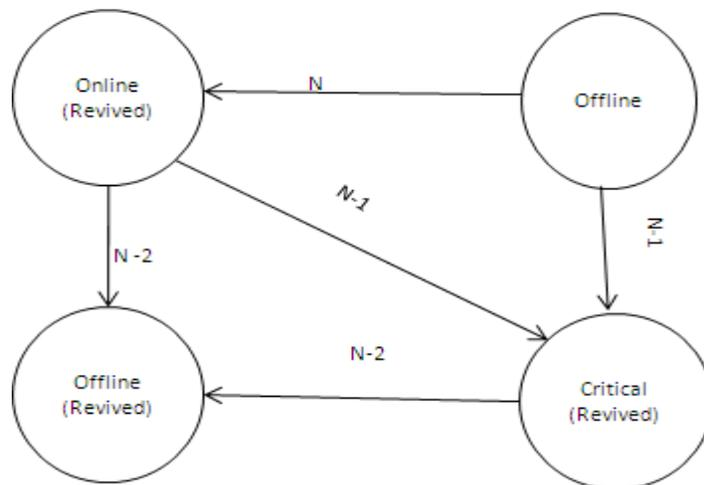
Logical Array State Diagram – Redundant RAID Level RAID 5EE
