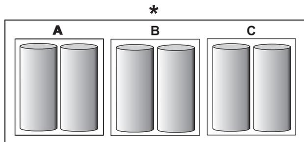
A sub-logical drive is created within *each* logical drive (A, B, and C). Then, the data is striped across the physical drives, creating blocks.
