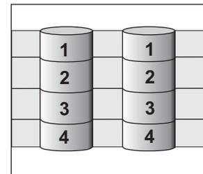
With RAID level-1, if one of the physical drives fails, the controller switches read and write requests to the remaining functional drive in the RAID level-1 logical drive.
