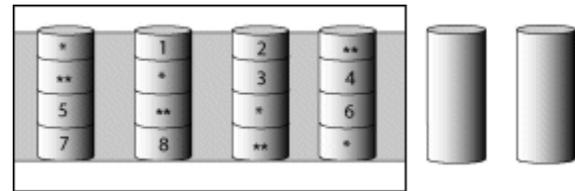
The storage of the data parity (denoted by \* and \*\*) is striped, and it shifts from drive to drive as it does in RAID level-5.
