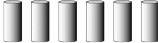
Create a logical drive using four physical drives, leaving two drives for data parity.
