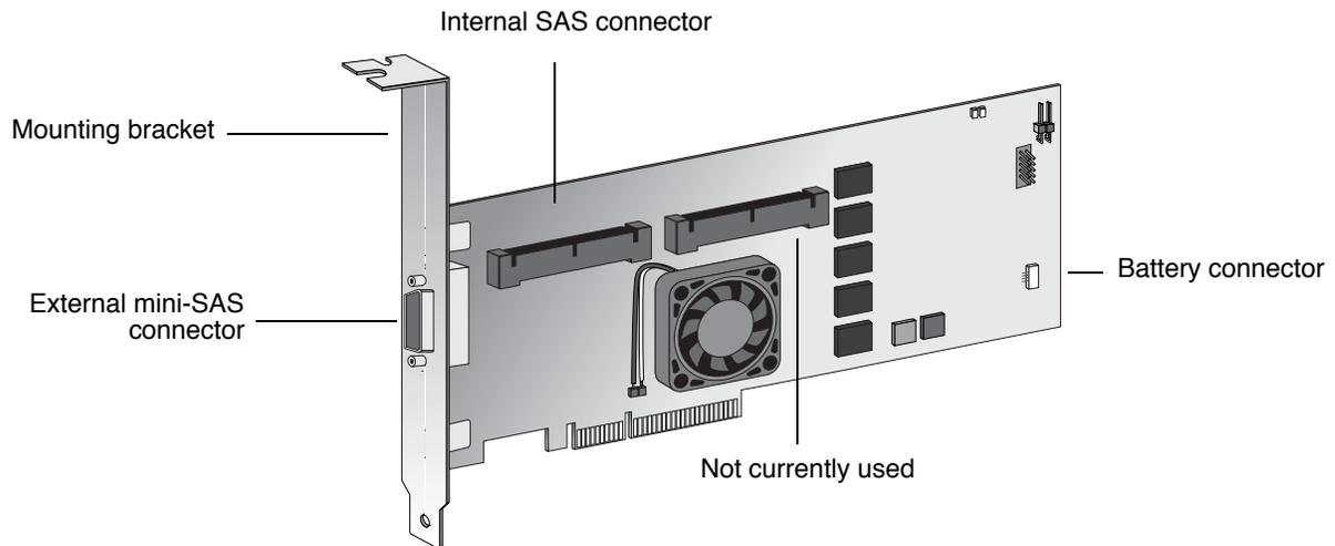
**Note:** The ServeRAID-8s controller has the option for a backup battery module containing a lithium battery. (The part number for the optional backup battery module is IBM Part Number 39R8765. However, if you replace the battery, you should order replacement battery IBM Part Number 13N2256.)
