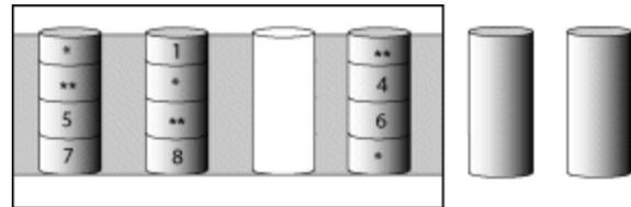
If a second physical drive fails in the logical drive, the data from both failed drives is reconstructed onto the data parity drives, and the data for the logical drive returns to the original striping scheme.
