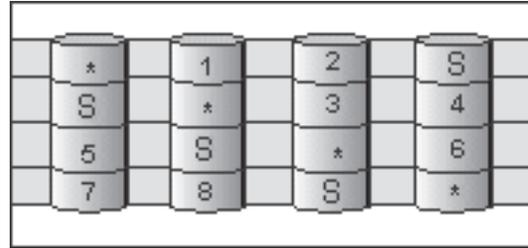
If a physical drive fails, the data from the failed drive is reconstructed. The logical drive undergoes compaction, and the distributed spare drive becomes part of the logical drive. The logical drive remains RAID level-5EE.
