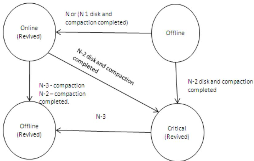
Logical Array State Diagram – Redundant RAID Level RAID 6
