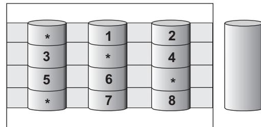
A parity block (\*) contains a representation of the data from the other blocks in the same stripe. For example, the parity block in the first stripe contains data representation of blocks 1 and 2.
