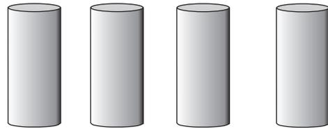
Create a logical drive using three of the physical drives, leaving the fourth as a hot-spare drive.
