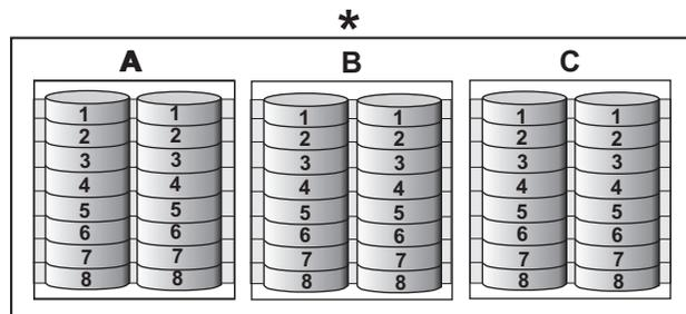
Then, create a logical drive within the spanned logical drive (\*). The data is striped across this logical drive, creating blocks (1-12). Notice that none of these blocks are redundant. This is because the logical drive is RAID level-0 in a RAID level-x0 implementation (see the following table).
