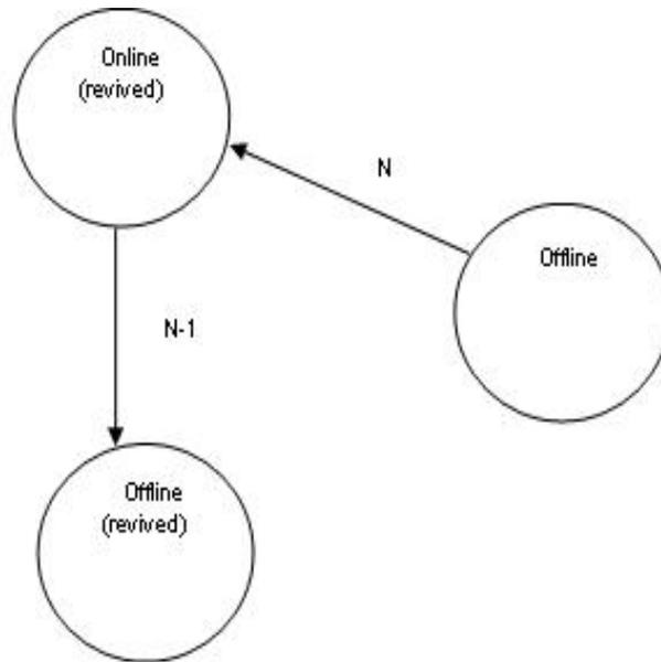
Logical Array State Diagram– Redundant RAID Level (RAID 5,1,1E,10,50)
