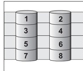
A physical drive failure within the logical drive results in loss of data in the logical drive assigned RAID level-0, but only in that logical drive. Logical drives assigned RAID level-1, level-1E, level-5, level-5EE, or level-6 do not lose data.
