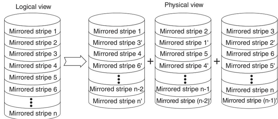
The controller has a BIOS-based configuration utility. This utility enables you to create integrated mirroring and integrated mirroring enhanced volumes during initial setup and to reconfigure them in response to hardware failures or changes in the environment.
