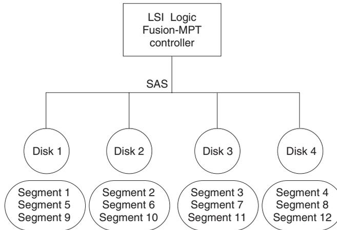
The following illustration shows a logical view and a physical view of an integrated striping configuration.
