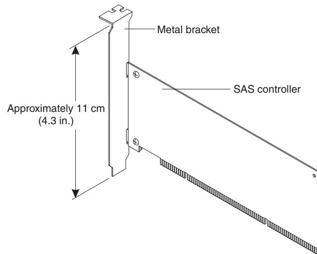
The option package also contains a low-profile expansion-slot bracket that is approximately 7 cm (2.9 in.) long. If the opening for the PCIe expansion slot is approximately 6 cm (2.3 in.) long, you must replace the preinstalled bracket with the low-profile bracket. You will do this in step 5 in the following procedure.
