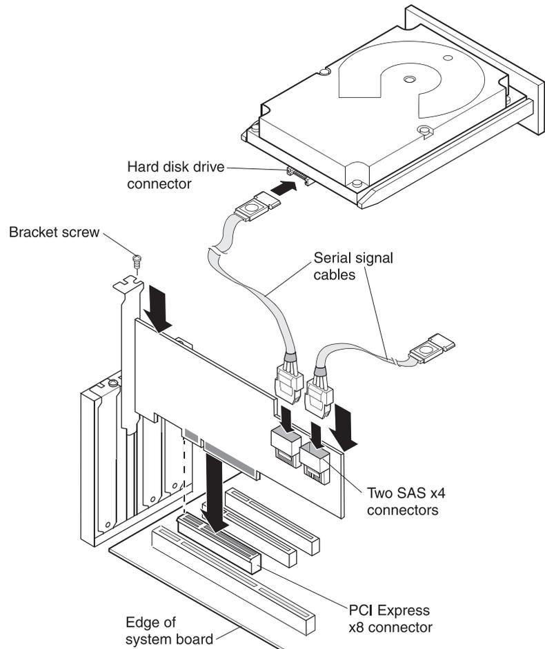
8. Replace the expansion-slot cover to secure the controller to the server chassis. Replace the expansion-slot screw if you removed it in step 6 on page 10.
