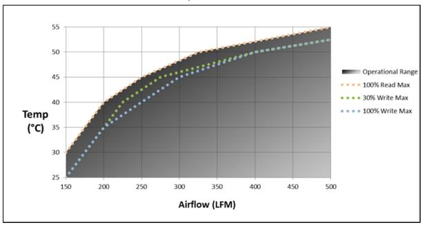
Where the temperature is the **ambient temperature** of the air, in °C, as it comes in contact with the device. For example, if your inlet temperature to the device was 48 °C, you would need airflow of at least 300 LFM in order to operate the device at 100% reads.
