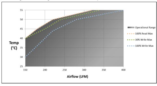
Where the temperature is the **ambient temperature** of the air, in °C, as it comes in contact with the device. For example, if your inlet temperature to the device was 48 °C, you would need airflow of at least 220 LFM in order to operate the device at 100% reads.
