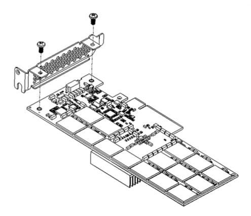
5. Attach the half-height bracket using a Phillips #1 tip screwdriver to tighten the two screws.
