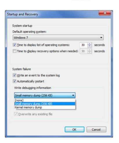
In the System Failure section you can change settings to handle the system log, restart, and debugging information.
