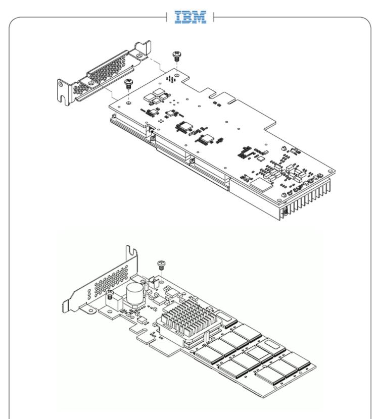
5. Attach the half-height bracket using a Phillips #1 tip screwdriver to tighten the two screws.
