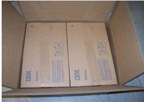
2.2.3 Once the Blades are secure in the multipack carton, close the flaps of the carton (44R3910) and seal with specified tape.
