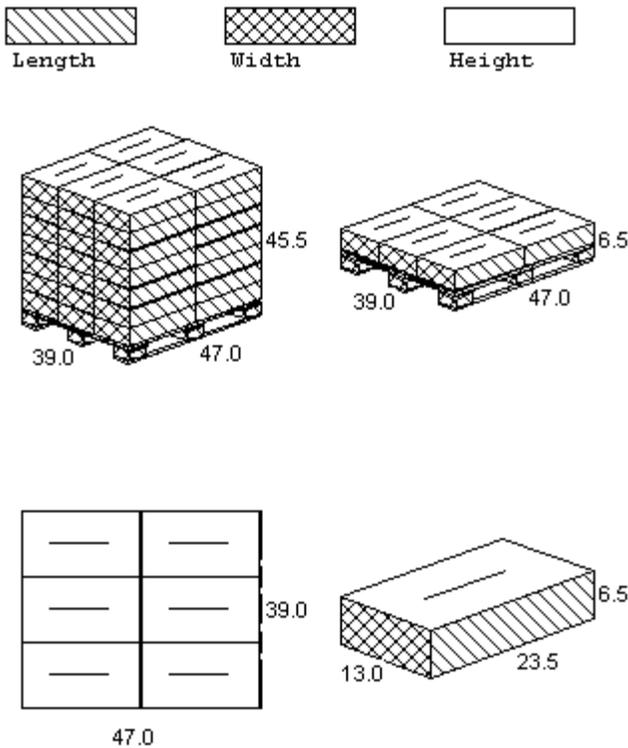
2.3.2 - Secure load to pallet utilizing "Best of Breed" palletization methods. See 92F6168 - "Best of Breed" Pallet Unitization or QMX document P-04146.
