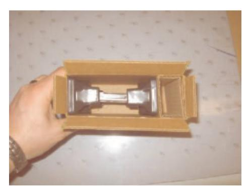
**2.5** - Grab for pubs, ensure the pubs are folded in half top to bottom, then slide the pubs down in between the carton side wall and the HDD.
