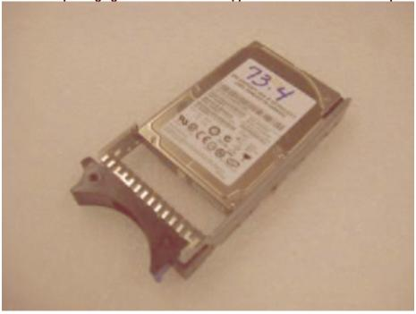
**1.0** - Assemble 2.5" HDD and packaging, then seal the bottom of the RSC P/N 46D2050 shut with IBM logo tape P/N 46D2114.
