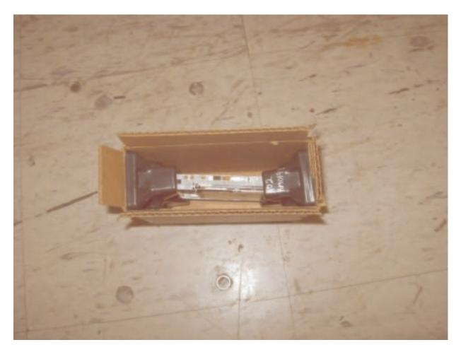
1.5 - Grab for pubs, ensure the pubs are folded in half top to bottom, then slide the pubs down in between the carton side wall and the HDD.
