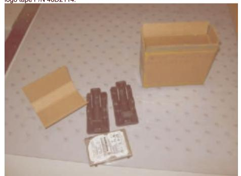
2.1 - Place HDD assembly in ESD P/N 4759223, fold bag and seal opening with ESD label P/N 6937292.
