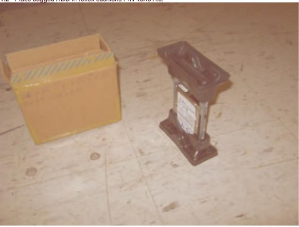
1.3 - Place HDD assembly in to carton P/N 46D2050.
