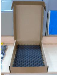
2.3 - Center the supplier prepared bagged parts into the box as shown.
