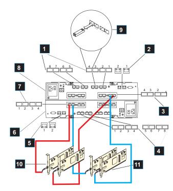
1 and 4 2 and 5 Ethernet ports Host ports 3 and 7 Controller B Controller A Host 1, host adapters 1 and 2 Host 2, host adapters 1 and 2
