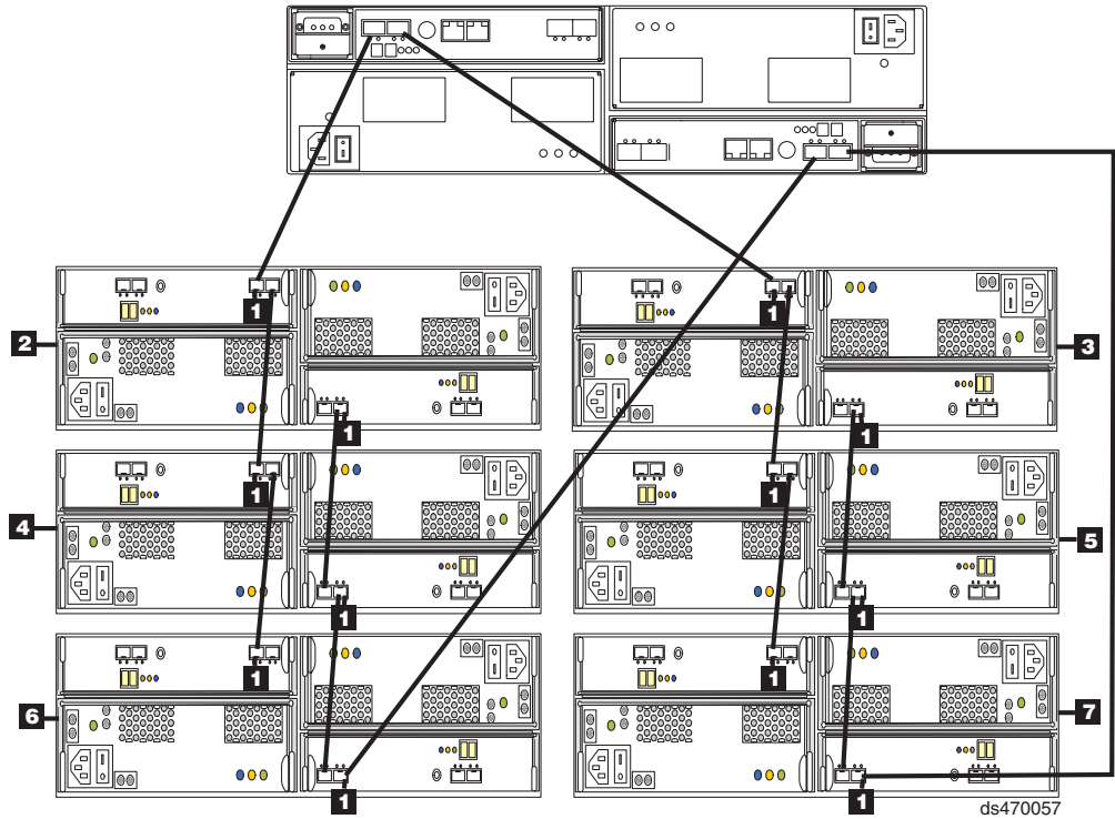
Figure 51. One DS4200 Express and a maximum of six EXP420 storage expansion enclosures behind a pair of DS4200 Express drive ports
