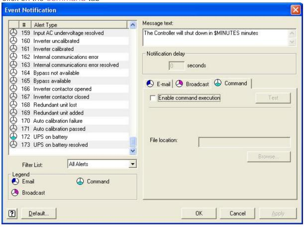
7. Tick the box left to *Enable command* execution and enter the path to the script file
