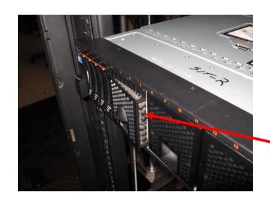
Note that after shipment of a 7148/7149 system configured in a rack. The SSD bezel may come loose (as shown here). To reinstall, simply push back into place.
