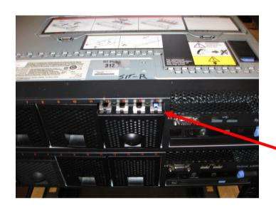
Note that after shipment of a 7148/7149 system configured in a rack. The Simple Swap HDD bezel may come loose (as shown here). To reinstall, simply push back into place.
