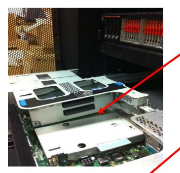
Improper install method. The card should not be installed on an angle.
