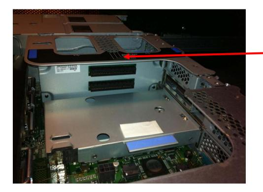
Proper method for installing the card is to hold it flat and push it straight down into the planar connector.
