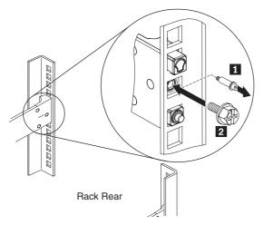
To secure the server or memory expansion module in a rack, complete the following steps:
