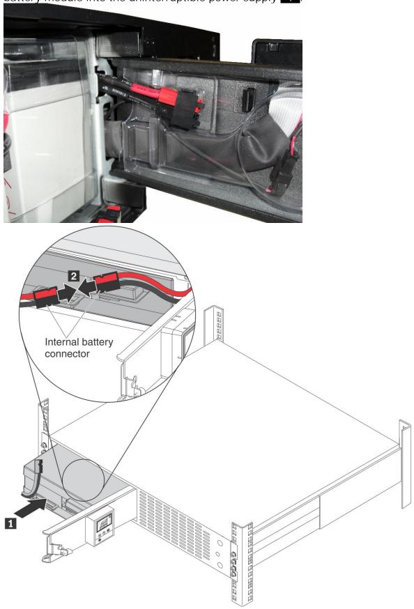
8. Connect the internal battery connector 2 - see graphics on previous page for more details - after pulling it out of the holder in the cover door with the connector on the battery.
