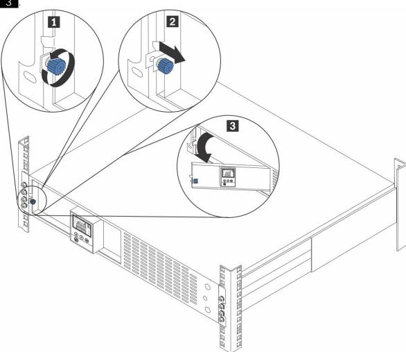
3. Disconnect the internal battery connector 1 and move connector on the battery out of the way and place the internal connector into the holder in the cover door.
