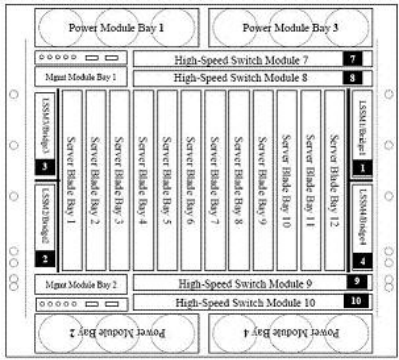
Figure 2. BladeCenter HT DC (8740) rear view
