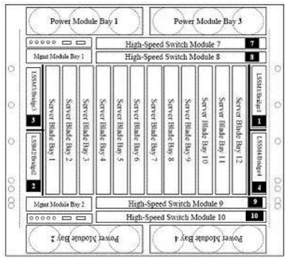
Figure 2. BladeCenter HT AC (8750) rear view
