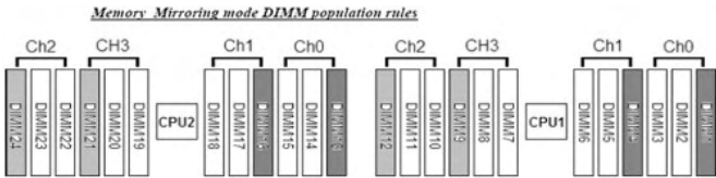
Figure 2. System 3650 M5 (5462) Memory Mirroring mode DIMM population rules
