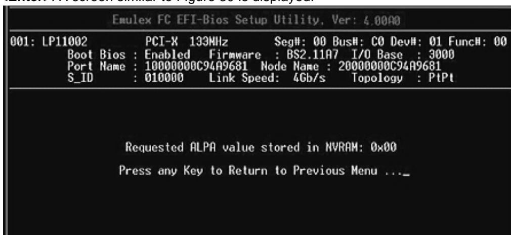
Figure 30: Default AL_PA Setup screen
