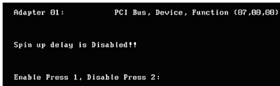
Figure 13: Enable or Disable Spinup Delay screen
