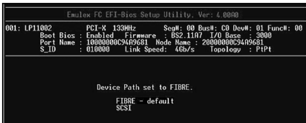
Figure 35: Device Path screen
