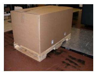
**2.20** Print and place carton labels on label tick marks located on carton. Reference QMX document SG-P-01486 "Special Packaging Labeling Guidelines" which may contain additional labeling requirements.
