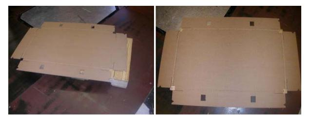
**2.5** Attach PBJ tray (22K8090) to pallet using a minimum of eight staples (22K8096) as shown.
