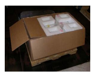
**2.19** Close the top of the carton and seal with tape. For IBM branded units, use IBM logo tape: 46D2114 (manual) or 46D2115 (automatic) For OEM blank carton units, use clear tape: 6272199
