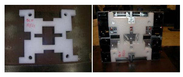
**2.4** Align PBJ tray (22K8090) with half pallet (PN varies by site). Use windows and alignment marks to help center the tray.
