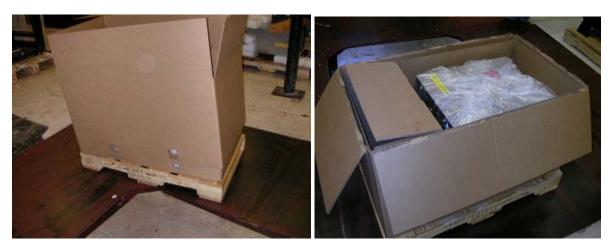
**2.16** Attach carton to tray/pallet assembly using four corrugated clips (37L0511).
