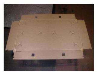
2.6 Use Sanstrap (37L7558) to set up tray as shown below. The notches on each flap will help hold Sanstrap in place.
