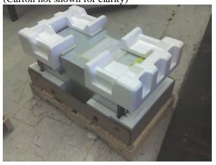
\*\*\*2.18b Locate two top fabricated cushions (44R3960), and place on top of unit.
