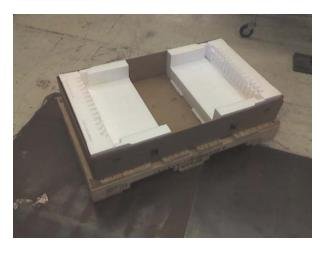
\*\*\*2.6b Locate two bottom fabricated cushions (44R3959) and two fabricated inserts (44R3958) in preparation for placing in tray. Make sure they are set up correctly as shown below.
