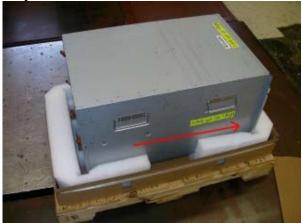
**2.11** Apply a 2 inch (50mm) strip of appliance tape (01R3747) to each of the four handles to hold them in the down position.
