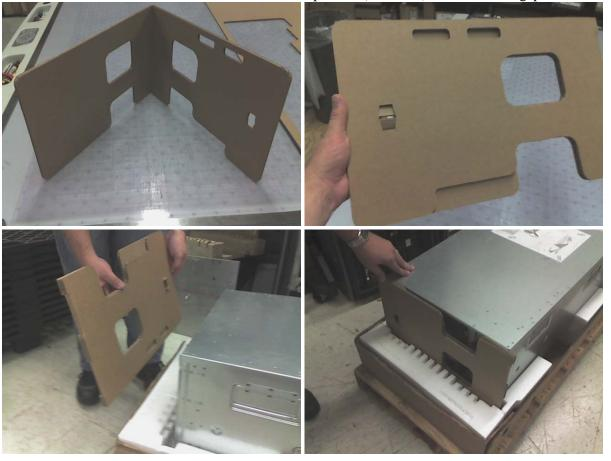
2.14 Locate PBJ carton (44R3990 - IBM, 22K8111 - OEM) and fold bottom panels into carton, ends first.
