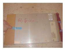
1.3- Place the Blade in ESD bag 37L8109, as shown below, and seal it closed using Padlock Tamper Seal 06P6550..
