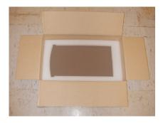
1.6- The Blade is placed into the middle of the PE Cushion 22K8230 with the Bezel facing curved section of cushion. The Blade must ship with the ESD Bag , the second picture is just to ensure proper orientation .
