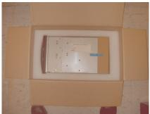
1.7- Remaining Urethane Cushion 22K8229 is placed on top of Blade. Top U-Tray 22K8231 is set on top of Cushion.
