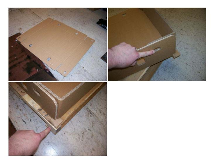
1.4 Attach PBJ tray (43X3215) to pallet using a minimum of eight staples (22K8096) as shown.
