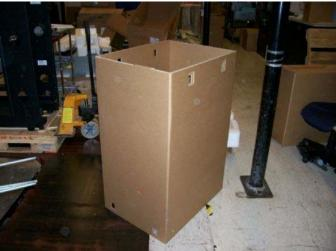
1.14 Place assembled carton (43X3213 - IBM or 44R3975 - OEM) over system and tray (NOTE: carton sits on the pallet outside the tray).
