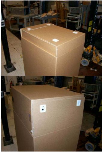
A4. Place tamper label (74F8851) over two clips holding shipgroup to system carton.
