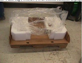
**1.8** Place unit in bottom cushion. Make sure the system is fully seated in the cushions. The front of the system is the flat face of the cushion. The notched side is for the rear.
