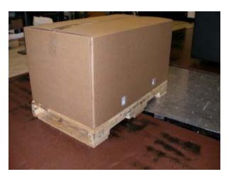
**1.21** Print and place carton labels on label tick marks located on carton. Reference QMX document SG-P-01486 "Special Packaging Labeling Guidelines" which may contain additional labeling requirements.
