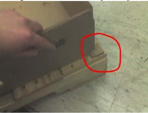
**2.**5 Attach BladeCenter pallet tray (44R3952) to pallet using a minimum of eight staples (22K8096) as shown. (NOTE: old style tray shown in picture. Staple location should remain the same.)
