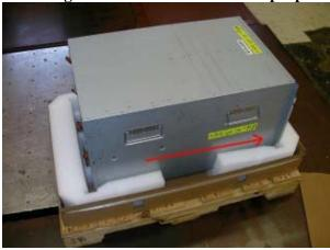
**2.12** Apply a 2 inch (50mm) strip of appliance tape (01R3747) to each of the four handles to hold them in the down position.
