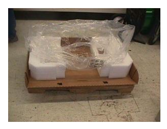
**2.11** Place unit in bottom cushions. Make sure the system is fully seated in the cushions and placed all the way forward. There will be a  $\sim$ 1" gap behind the system.
