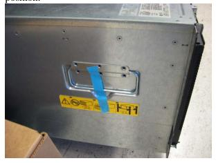
**2.13** Making sure bag is pulled tight, use Tamper Label (06P6550) to seal edges of bag closed.
