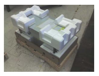
\*\*\*2.21b Locate two universal fabricated cushions (44R3950), and place on top of unit.
