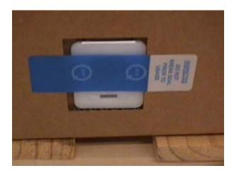
NOTE: Fabricated cushion alternate method below in 2.21b. 2.21 Place two top cushions on top of system as shown. (Carton not shown for clarity)
