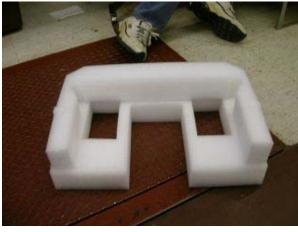
\*\*\*2.7b Place cushions in tray making sure that the cushions are placed all the way to the front and rear of the tray (as shown).
