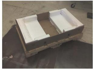
\*\*\*2.6b Locate two universal fabricated cushions (44R3951) in preparation for placing in tray. Make sure they are set up correctly as shown below.
