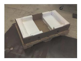
\*\*\*2.6b Locate two universal fabricated cushions (44R3950) in preparation for placing in tray. Make sure they are set up correctly as shown below.
