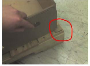
2.5 Attach BladeCenter pallet tray (44R3952) to pallet using a minimum of eight staples (22K8096) as shown. (NOTE: old style tray shown in picture. Staple location should remain the same.)
