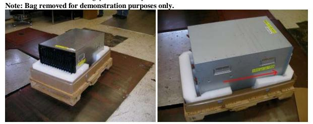
2.11 Apply a 2 inch (50mm) strip of appliance tape (01R3747) to each of the four handles to hold them in the down position.
