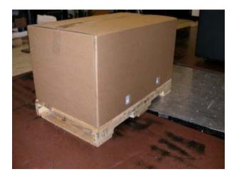
2.24 Print and place carton labels on label tick marks located on carton. Reference QMX document SG-P-01486 "Special Packaging Labeling Guidelines" which may contain additional labeling requirements.
