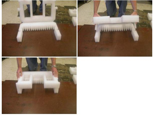
\*\*\*2.7b Place cushions in tray making sure that the cushions are placed all the way to the front and rear of the tray (as shown).
