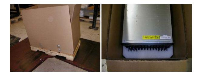
2.16 Attach carton to tray/pallet assembly using four corrugated clips (37L0511).
