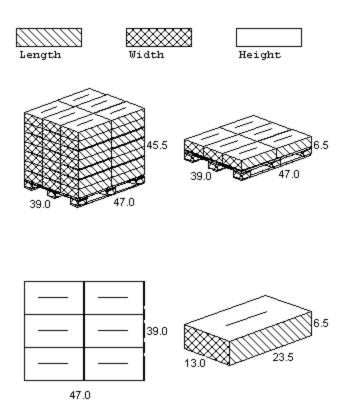
2.1.2 - Secure load to pallet utilizing "Best of Breed" palletization methods. See 92F6168 - "Best of Breed" Pallet Unitization or QMX document P-04146.
