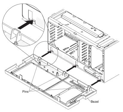
2) Rotate the bezel toward the server and press until it snaps into place.
