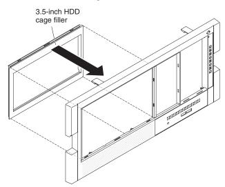
b) Attach the 3.5-inch drive ID label on the bezel.
