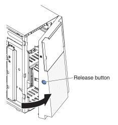
3. Pull the hinge assemblies upward and release the bezel out of the chassis.
