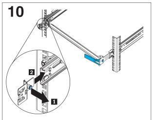
Install the cable management arm mounting bracket.
