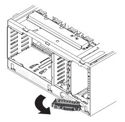
c. Squeeze the sides of the USB connector and remove it from the angled assembly. To install the flat assembly, squeeze the sides of the USB connector and connect it to the flat assembly.
