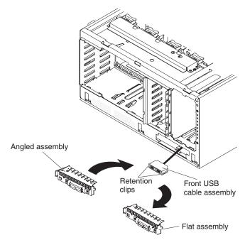
d. Use a flat-blade screwdriver to pry the holes on the angled assembly to release the light path diagnostics assembly. Remove the light path diagnostics assembly. To install the flat assembly, push the light path diagnostics assembly and secure it to the flat assembly.
