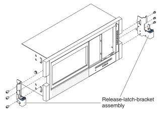
b. Secure the bracket with three M3.5 screws that come with this kit.
