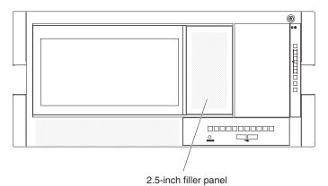
3) For models with 2.5-inch hard disk drives and 3.5-inch hard disk drives:a) Install the 3.5-inch cage filler.
