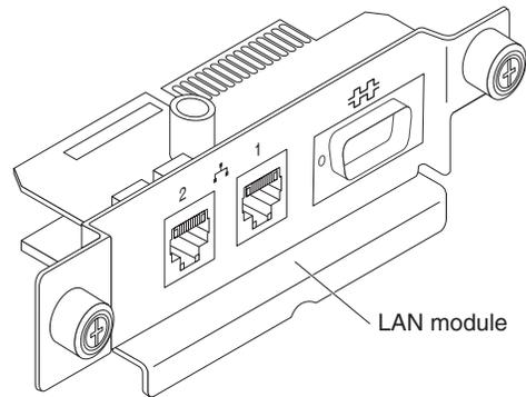
Use the instructions in this section to remove or install the LAN module into the rear of the BladeCenter T unit (see the illustration of the KVM and LAN modules in “Removing and installing the KVM (keyboard, video, mouse) module” on page 53). The LAN module is held in place by captive thumbscrews. You can use your fingers to turn the thumbscrews to install or remove the LAN module. Make sure that you do not overtighten the thumbscrews.
