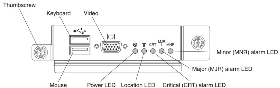
2. Position the KVM module into the rails inside the KVM-module bay.
