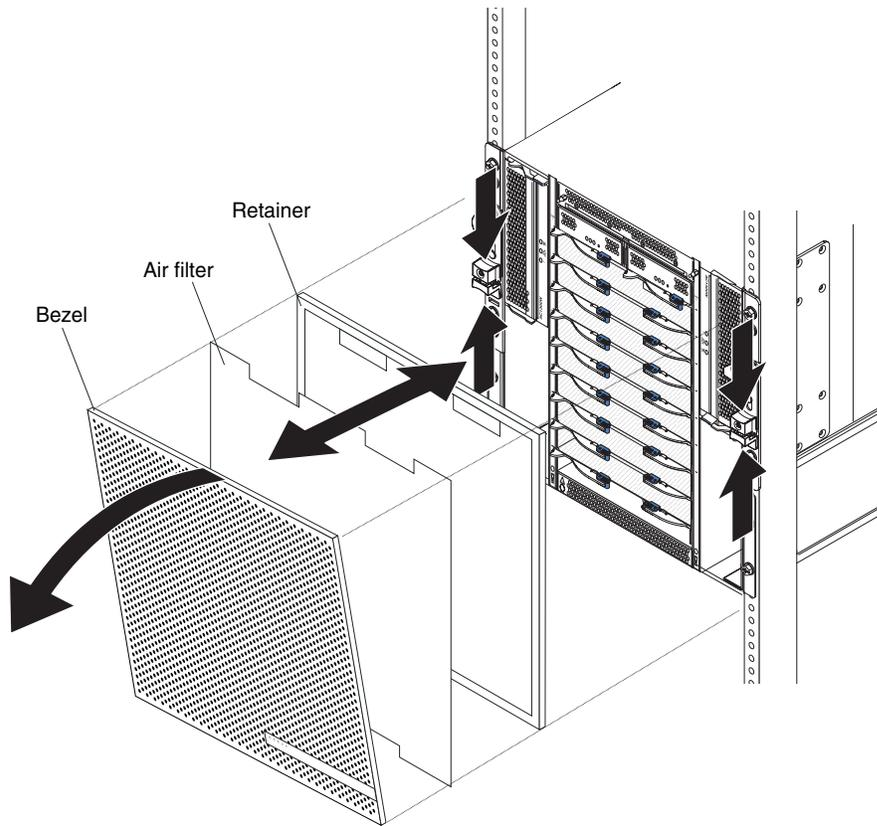
Complete the following steps to replace the front bezel air filter in the BladeCenter T unit:
