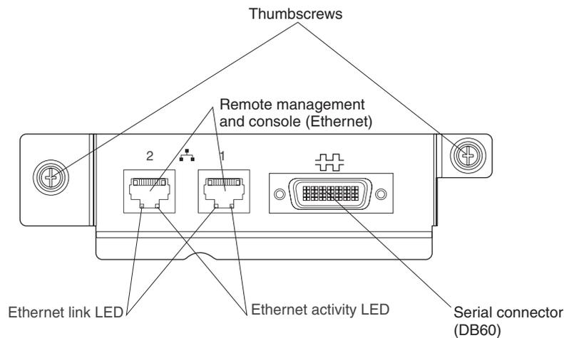
**LAN-module LEDs:** These LEDs provide status information about the LAN connection:
