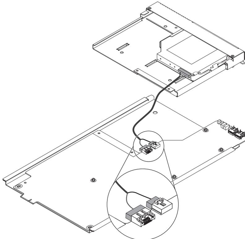
9. Connect the other end of the optical drive cable to the connector on the rear of the optical drive.
