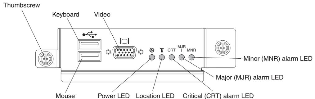
**System-status LEDs:** These LEDs provide status information for the BladeCenter T unit.
