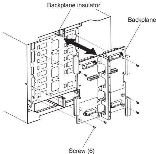
16. Holding the backplane at the top near the guide pins, pull the backplane out and off of the guide pins. Set the old backplane aside.
