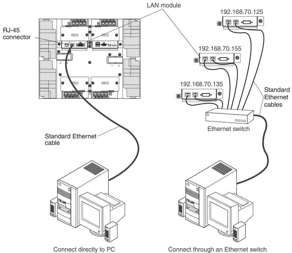
Complete the following steps to connect the Ethernet cable to the management module.
