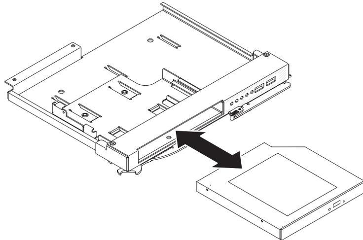
7. Attach the wire retention spring to secure the optical drive in the drive bay:
