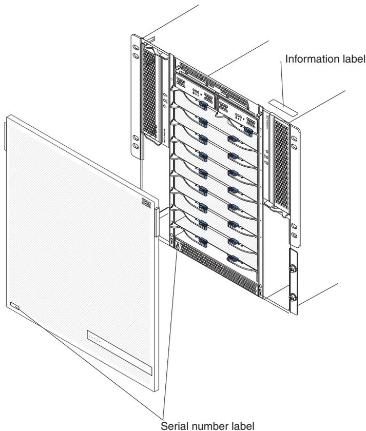
A set of user labels comes with each blade server. When you install a blade server in the BladeCenter T unit, write identifying information on a label and place the label on the BladeCenter T unit bezel.
