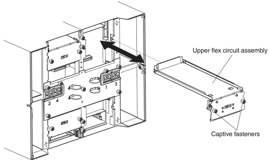
7. Carefully remove the old upper flex circuit assembly by placing your fingers under the lower edge of the assembly and pulling the unit out of the chassis.
