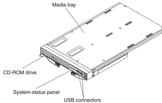
Use the instructions in this section to remove or install the media tray at the front of the BladeCenter T unit.
