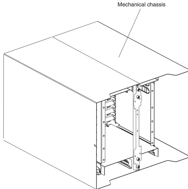
24. Install the backplane on the chassis; then, insert and tighten the six non-captive screws that mount the backplane to the chassis.
