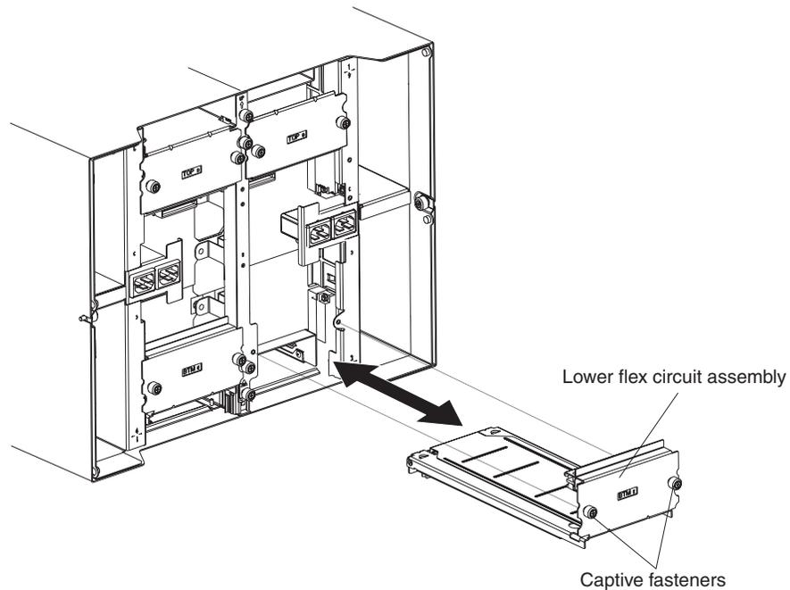
8. Carefully remove the old lower flex circuit assembly by gripping the top edge of the assembly and pulling the unit out of the chassis.
