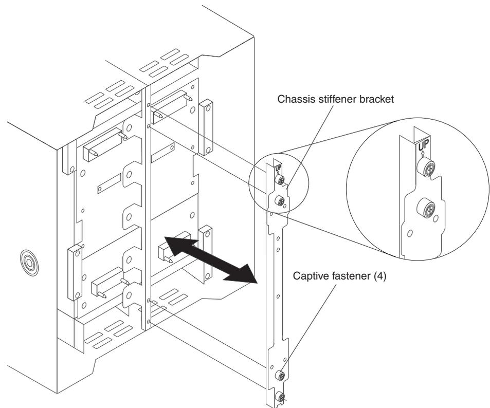
10. Pull the old rear chassis stiffener bracket off the chassis.
