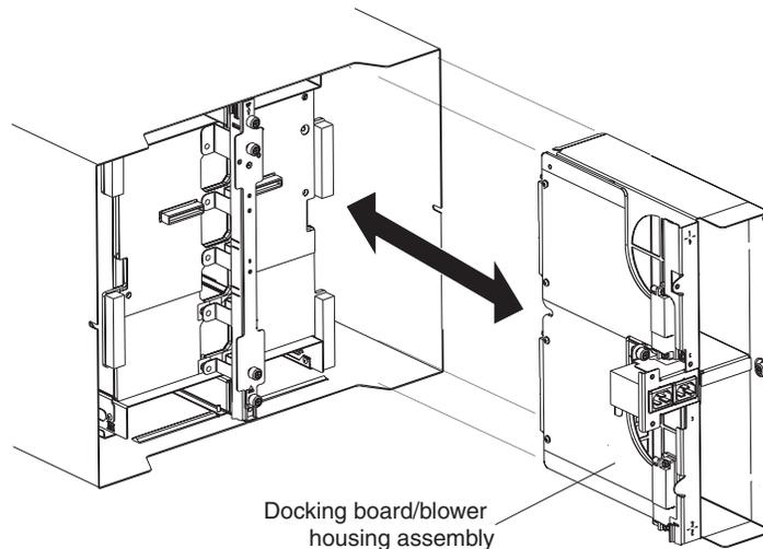
12. Grasp the housing by the housing frame above and below the power inlet receptacles, and carefully pull the housing out from the system chassis.
