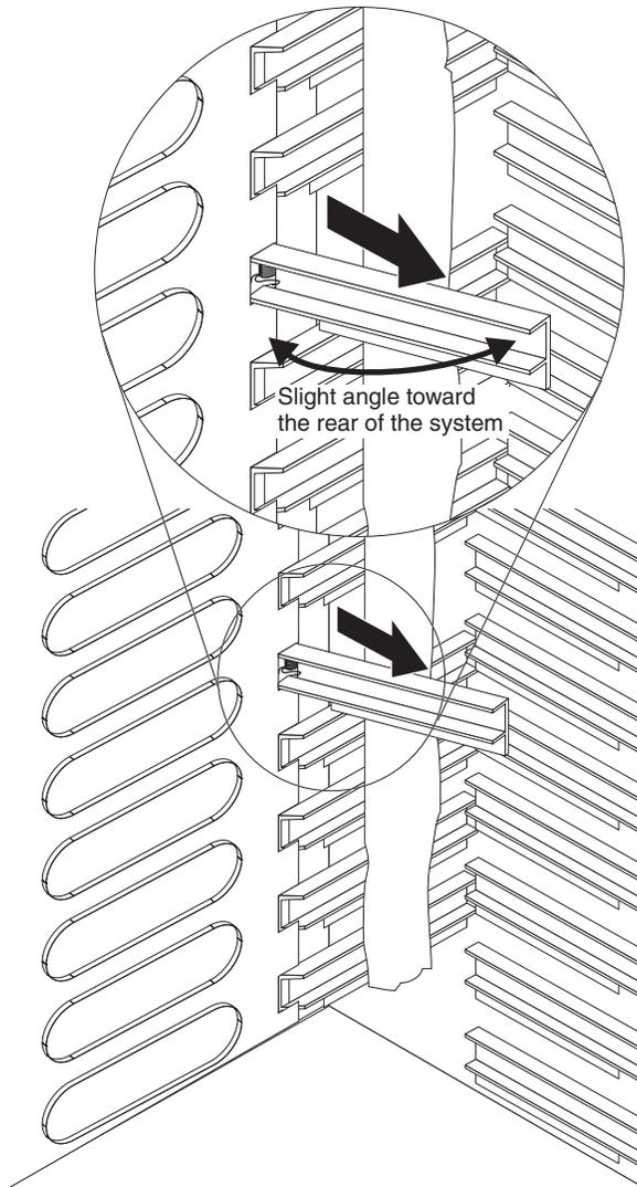
11. Hold the air damper angled slightly towards the back of the server; then, pull the air damper towards the center of the chassis until the pins on the air damper snap into the slots located on the back side of the air damper slot. Rock the air damper up and down while pulling on it to help it seat.
