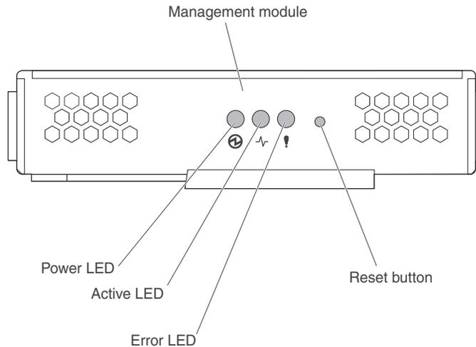
**Management module LEDs:** These LEDs provide status information about the management module and remote management connection.
