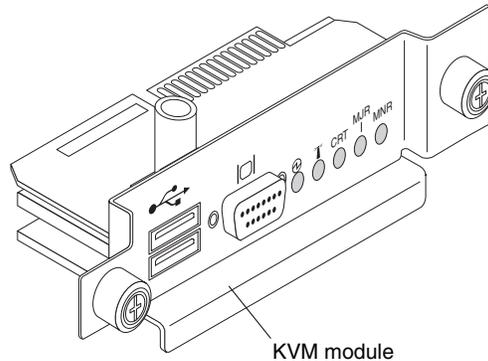
Use the instructions in this section to remove or install the KVM module from the rear of the BladeCenter T unit. The KVM module is held in place by captive thumbscrews. You can use your fingers to install or remove the KVM module. Make sure that you do not overtighten the thumbscrews.
