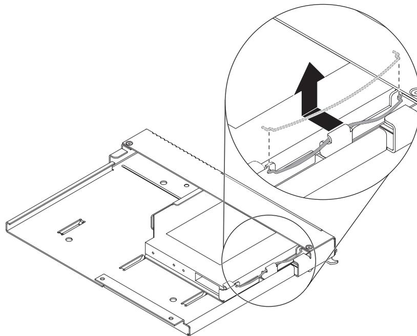
7. Slide the optical drive out of the drive bay.
