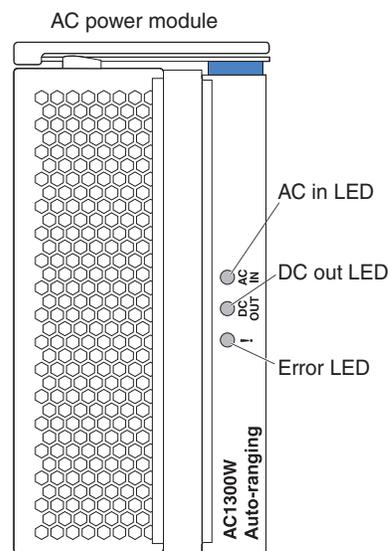
Make sure that the LEDs on the power modules indicate that they are operating correctly. Make sure that the input and output power LEDs on each power module are lit, and the error LEDs are not lit.
