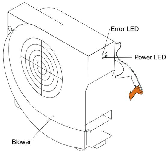
**Blower LEDs:** The LEDs on each blower provide status information about the blower.
