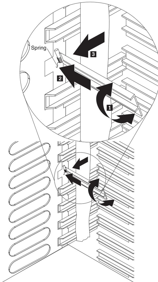
7. Use tape to hold the air dampers above and below the empty air damper slot in the open position. This will provide more room to install the air damper and reduce the chance of breaking additional air dampers.
