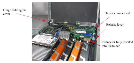
7. Lift up on the release lever until it is vertical.
