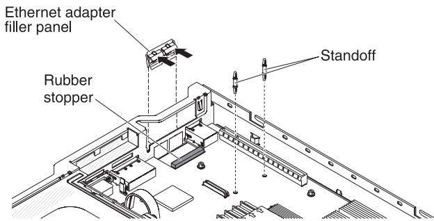
7. Install the two standoffs on the system board.
