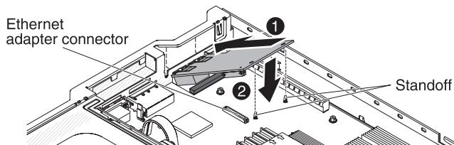
12. Slide the port connectors on the adapter into the port openings on the chassis; then, press the adapter firmly until the two standoffs engage the adapter. Make sure the adapter is securely seated on the connector on the system board.
