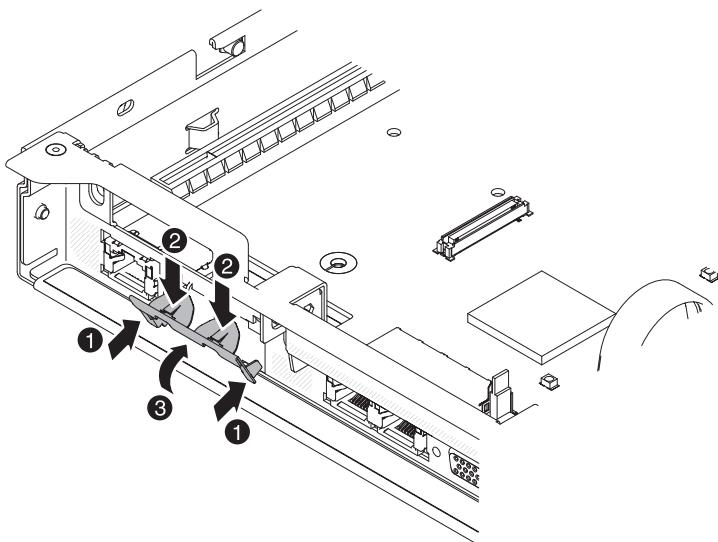
9. While you slightly press the top of the metal clip, rotate the metal clip toward the front of the server until the metal clip clicks into place. Make sure the metal clip is securely engaged on the chassis.
