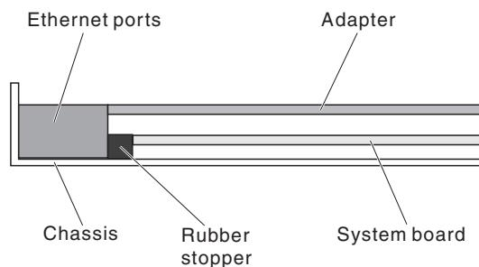
**Attention:** Make sure the port connectors on the adapter are aligned properly with the chassis on the rear of the server. An incorrectly seated adapter might cause damage to the system board or the adapter.
